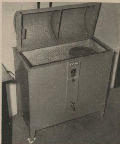
Figure 6.—A small combination electric water heater and utensil sterilizer available for small dairies. A three-gallon tank for heating water is located in the center of the cabinet. Note the design of the cabinet lid which provides vats for holding wash water.
