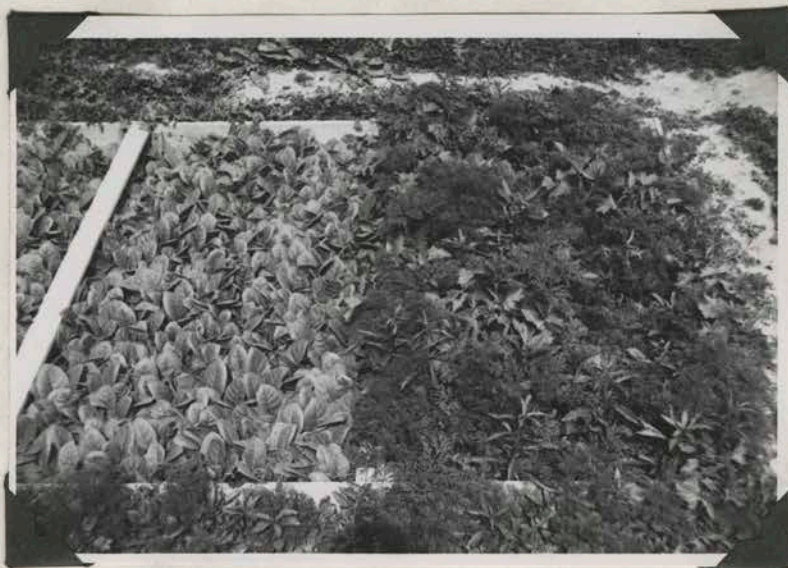
Results obtained in control of weeds by electric soil pasteurizer. Section of tobacco plant bed at left was pasteurized and section at right was not. Note dense growth of weeds in right side of bed.
