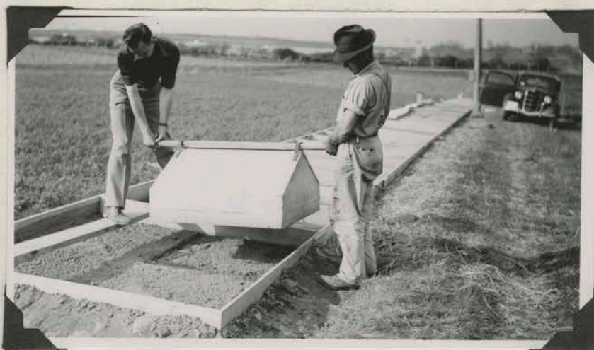
Electric Soil Pasteurizer developed in the agricultural engineering department and demonstrated in Washington County.
