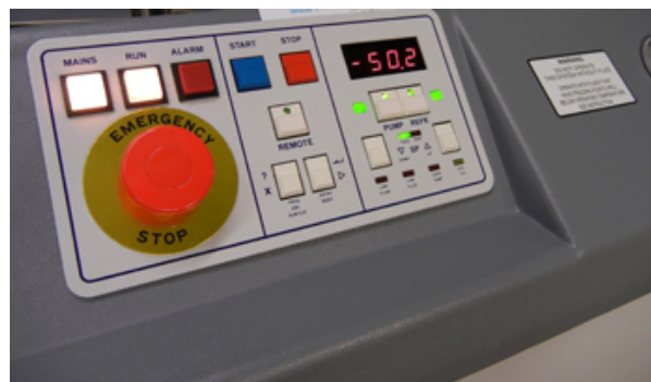
Figure 2.15: An IEC-compliant emergency-off button mounted on an industrial machine’s console [68].
