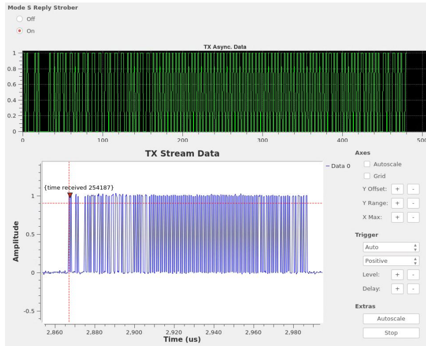
Figure 7.2: Real-time graphs of Figure 6.10 showing the DF 17 message received (and decoded in Figure 7.1).
