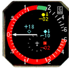
Figure 2.8: Example of a TCAS II traffic display with a “Climb 1500 ft/min” RA, as indicated by the square, red icon [58].
