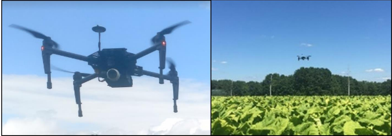
Figure 3.1- Matrice 100 quadcopter with Zenmuse X3 BGNIR camera being flown over the study area in the mid-season after topping has taken place. Flights were made at 50 meters above ground level.
