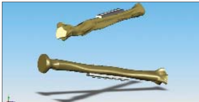
Figure 4. FE model of plated radius and ulna bones
