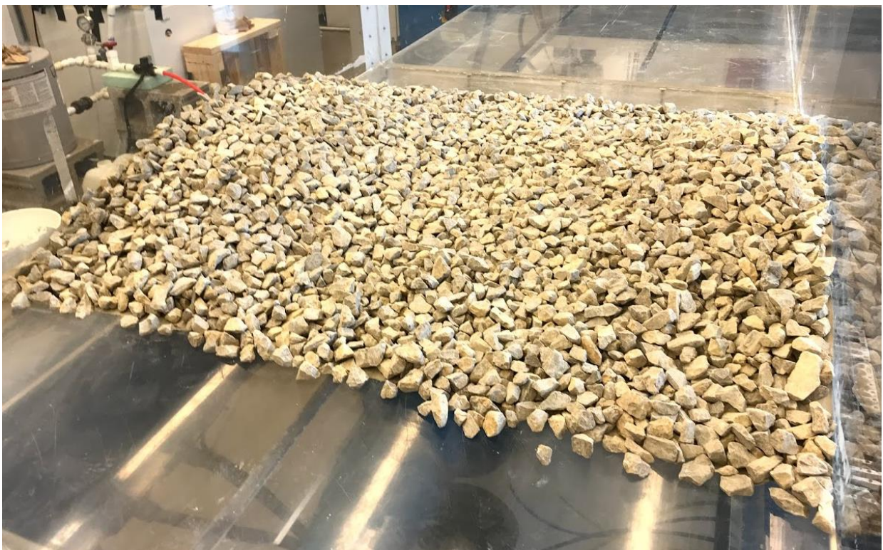
Figure 8. Completed rock weir configuration (Depth = 0.305 m (1.0 ft.), Length = 0.152 m (0.5 ft.), d_m = 12.7 mm (0.5 in.), bed slope = 0%).
