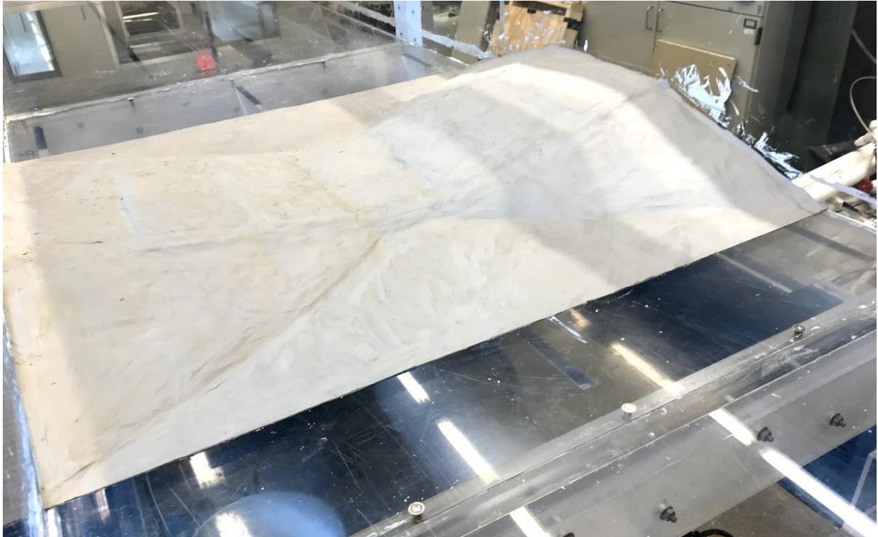
Figure 7. Rock weir core, constructed from porcelain clay. Configuration: depth= 0.305 m (1.0 ft.), length = 0.152 m (0.5 ft.), bed slope = 0%.
