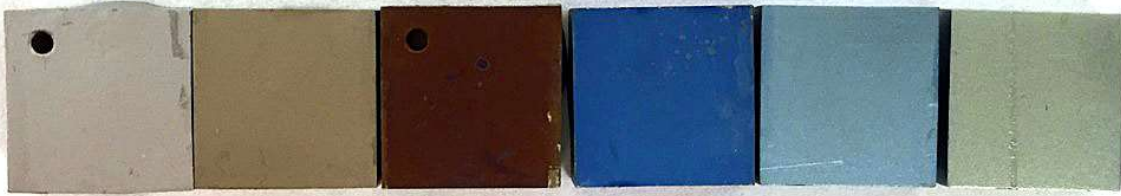
Figure B. 3 Anodized samples from left to right, Blank, 10V, 20V, 30V, 40V, and 50V.
