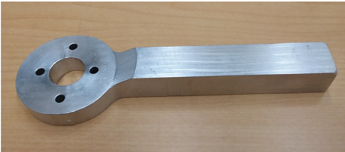
Figure 9.6: Custom motor mount for lathe testing to determine the thermal constant of the BLDC helicopter motors used in the prosthesis.
