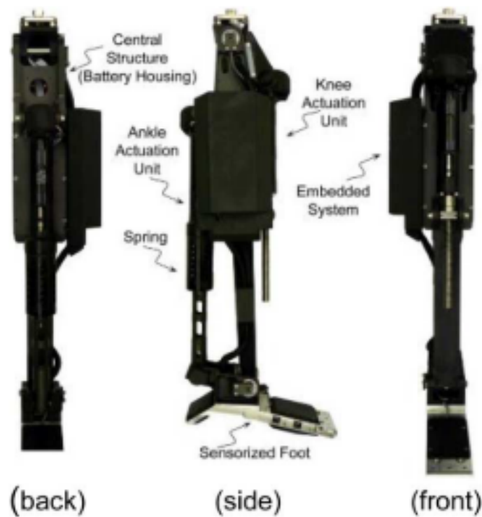
Figure 2.4: Vanderbilt Universities fully powered prosthetic leg for TFAs.
