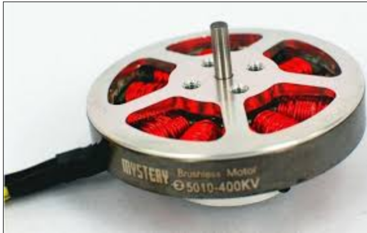
Figure 4.4: The Mystery hobby drone motor used for the ankle yaw degree of freedom.
