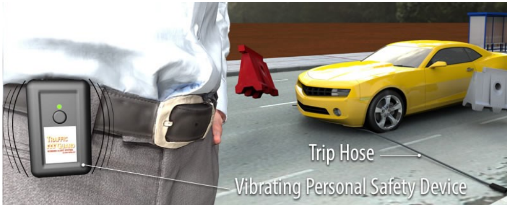
Figure 3. Traffic Guard Worker Alert System(Optics 2017)
