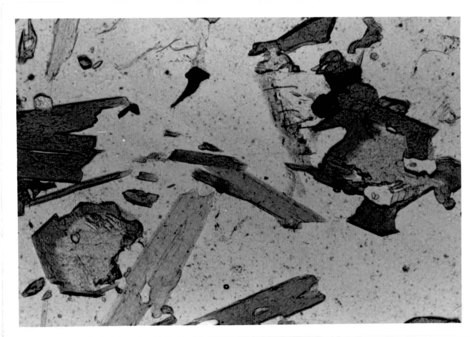
Figure 11: Photomicrograph of hornblende-rimmed anthophyllite surrounded by plagioclase and quartz in biotite-amphibole gneiss. Width of field: 1.1 mm.
