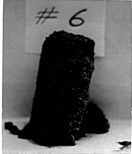
Figure 8. Specimen After Ten Cycles of Freezing and Thawing, Lime Content Seven Per Cent.
