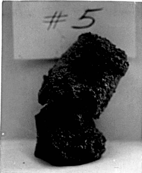
Figure 7. Specimen After Ten Cycles of Freezing and Thawing, Lime Content Zero Per Cent.
