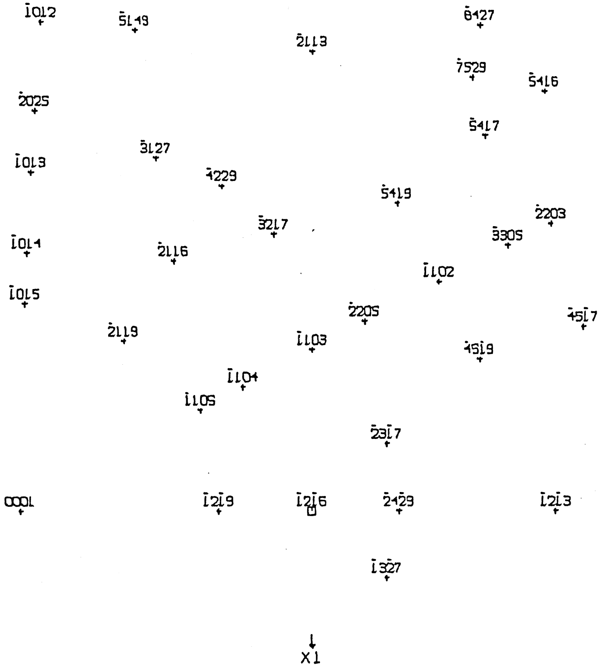
Fig. 53. [\bar{1}2\bar{1}6] zone projection associated with the Kikuchi projection shown in Figure 54. PSR = 25.00 cm, MDZP = 3, X_1 = [10\bar{1}0] .
