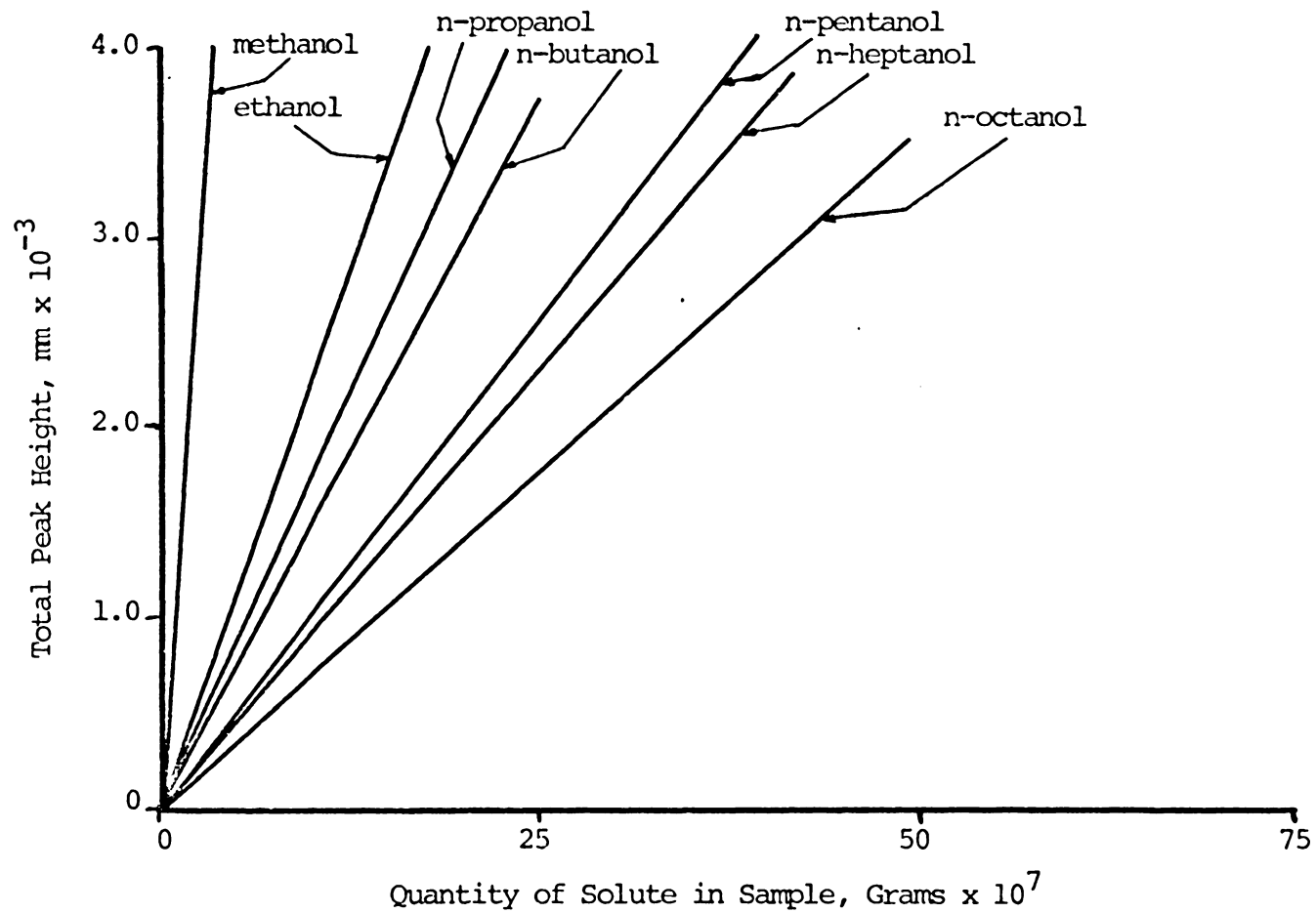
Figure 20. Response of the MAD as a Function of Quantity of Solute in Sample Adsorbent: Porous Glass Beads; Eluant: Benzene
