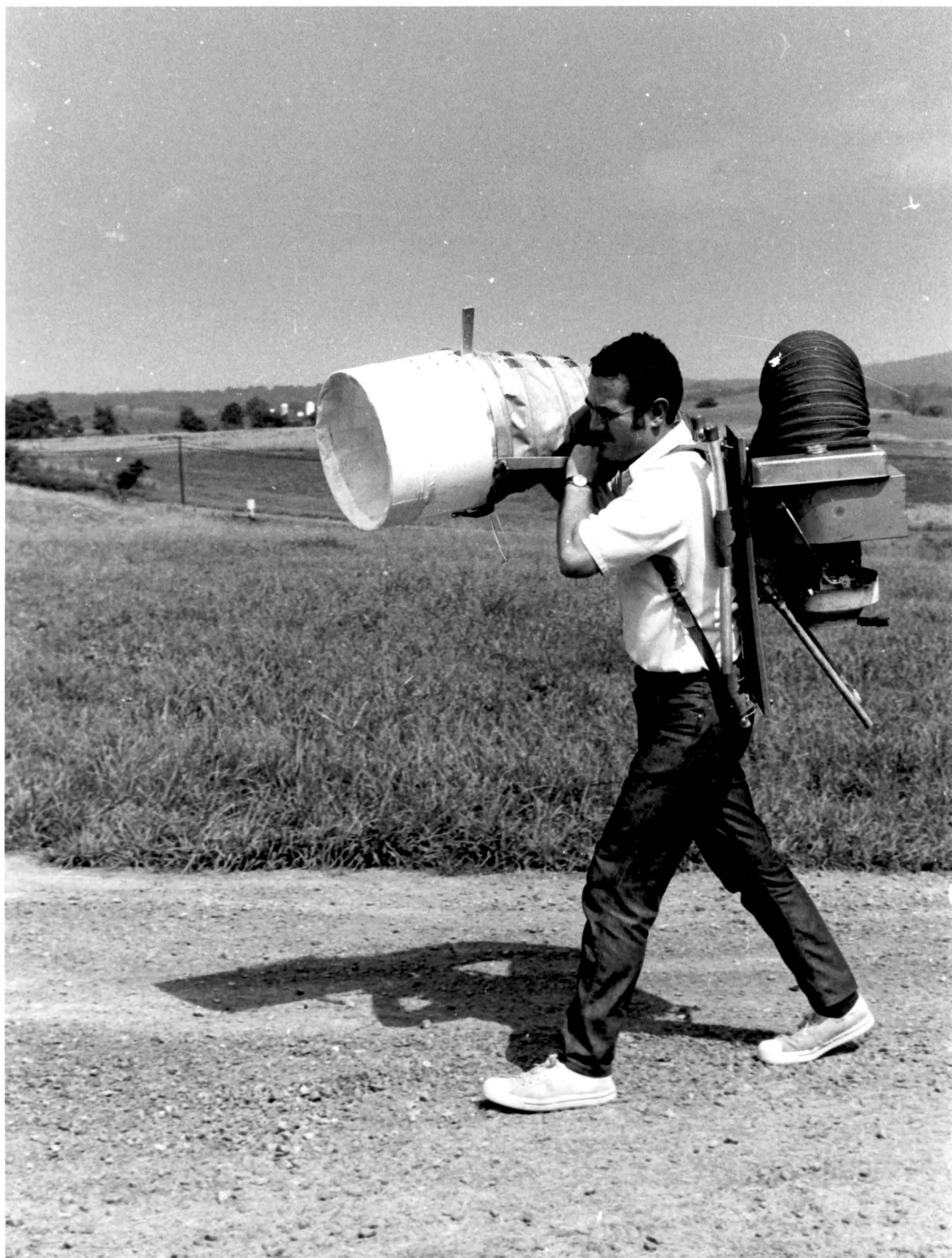
Figure 6. D-Vac Vacuum Insect Net used to sample the air for flying Culicoides spp.
