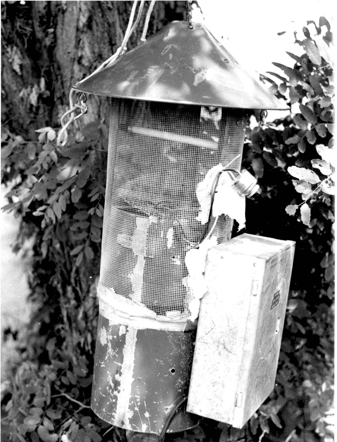
Figure 5. Standard New Jersey Light Trap converted for use as Black Light Trap.
