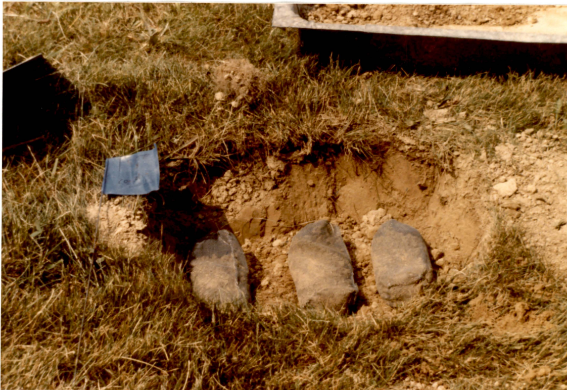
Figure 3.1. Mesh tubes filled with artificially infested soil and placed in the pit prior to burial.
