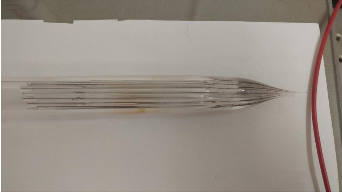
Figure 0-39: SiMF preform after drawing showing collapse of void space and draw down of features around core.
