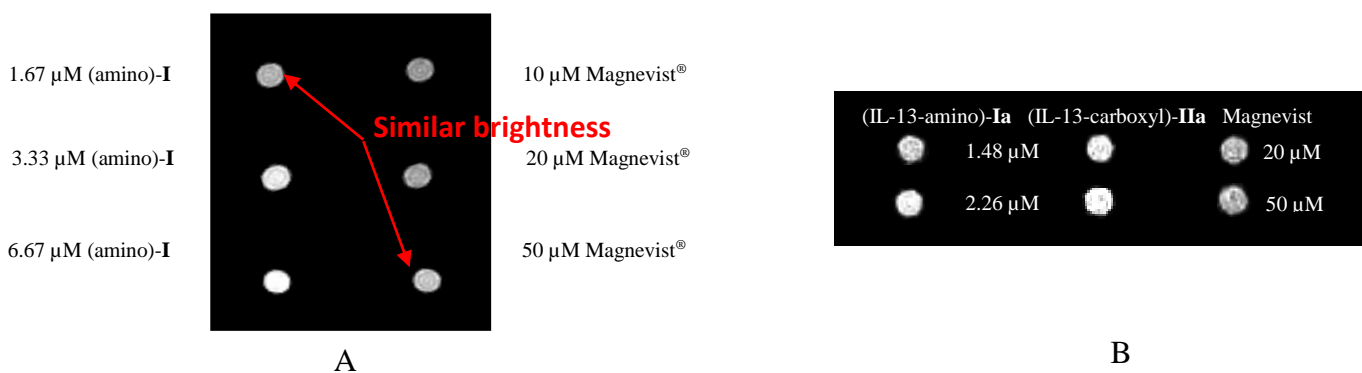
Figure 6. A) Inversion-recovery MR images ( T_I=1000 ms, T_R=5000 ms, T_E=30 ms) with (amino)- I and Magnevist ® as contrast agent. Left column from top to bottom: 1.67, 3.33 and 6.67 \mu\text{M} (amino)- I in water. Right column from top to bottom: 10, 20, 50 \mu\text{M} commercial agent Magnevist ® in water. The 1.67 \mu\text{M} (amino)- I and 50 \mu\text{M} Magnevist ® in water exhibit comparable contrast. B) Inversion-recovery MR images ( T_I=1000 ms, T_R=5000 ms, T_E=30 ms) with (IL-13-amino)- Ia and (IL-13-carboxyl)- IIa and Magnevist ® as contrast agent. The conjugated nanoparticles exhibit similar contrast with the commercial contrast agent.
