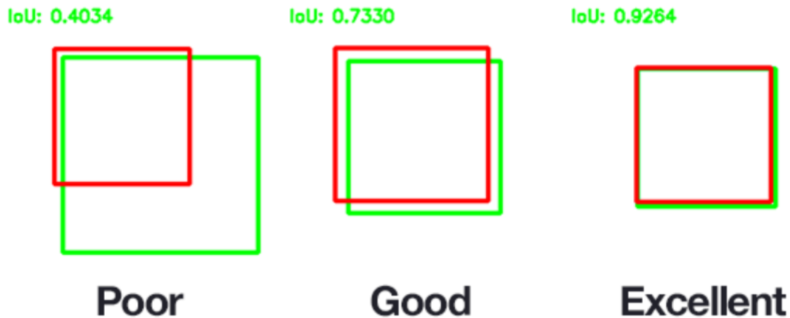
Figure 3.16: Relationship between the bounding boxes and IoU values[16]
