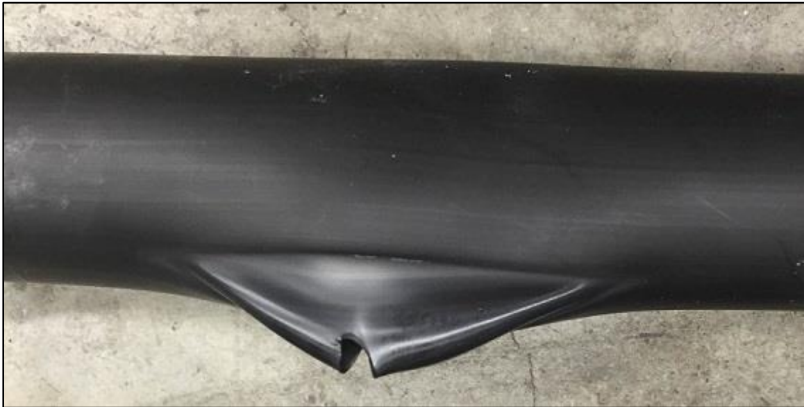
Figure 1: Ductile failure of an HDPE pipe.
