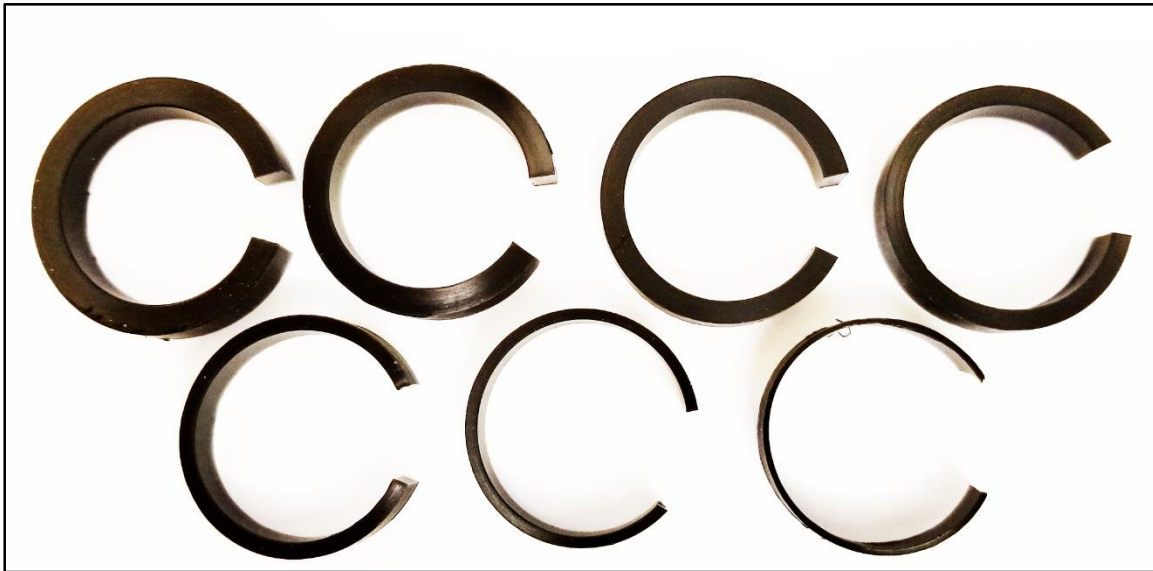
Figure 34: Prepared specimens for residual hoop stress measurements (the SDR 9 HDPE pipe).
