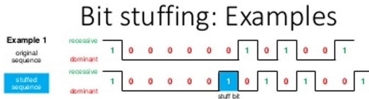
Figure 2.6: Bit stuffing in CAN bus frame for bit rate synchronization of CAN transceivers
