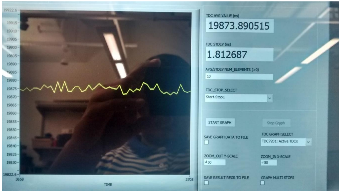
Figure 3.10: TDC measuring 19873 ns with a resolution of picoseconds
