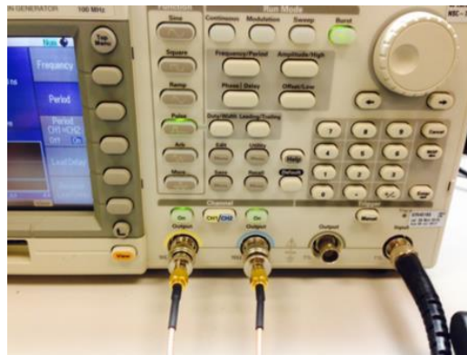
Figure 4.1: Physical connections to the TDC for start, stop and trigger pulses
