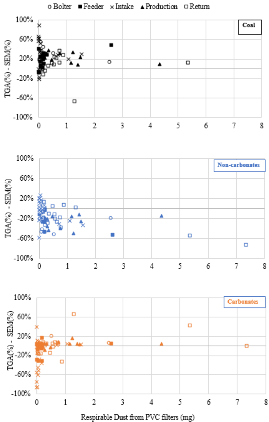
Figure B-3 Difference between TGA and SEM % vs dust weight (i.e., determined from PVC replicate filters) for a) coal b) non-carbonates and c) carbonates for key locations in underground coal mines
