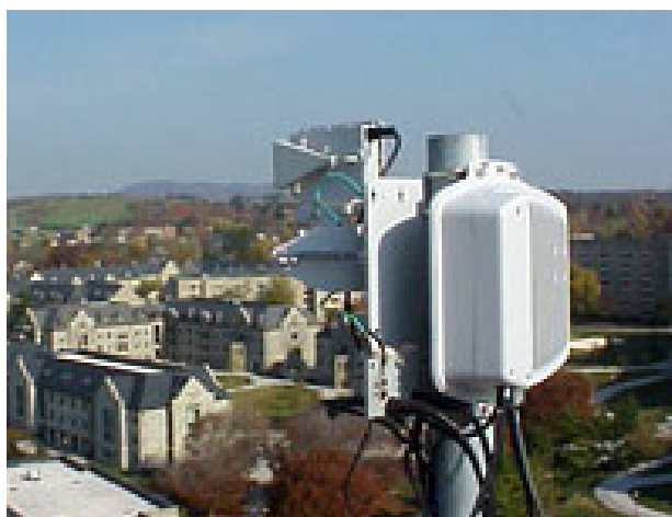
Harris-WavTrace LMDS multipoint hub deployed at Virginia Tech
