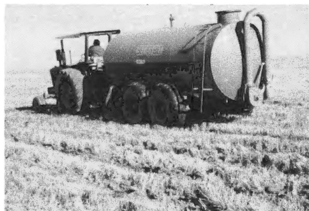
Figure 6. Injecting liquid wastes into the soil.
