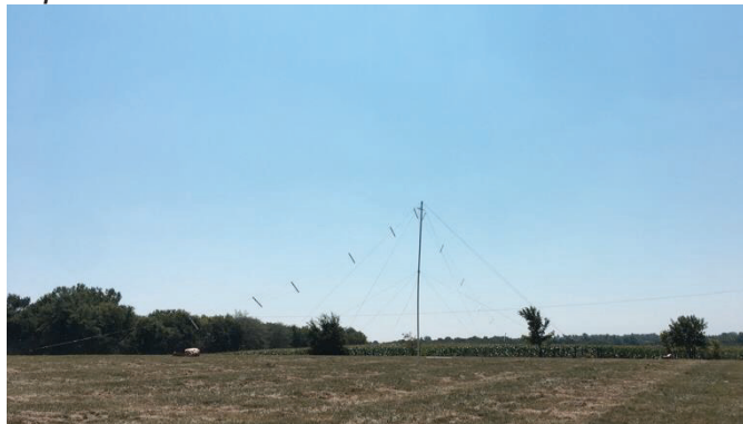
Figure 6. One of two fan dipole antennas for the ionospheric sounder in Holton, KS
