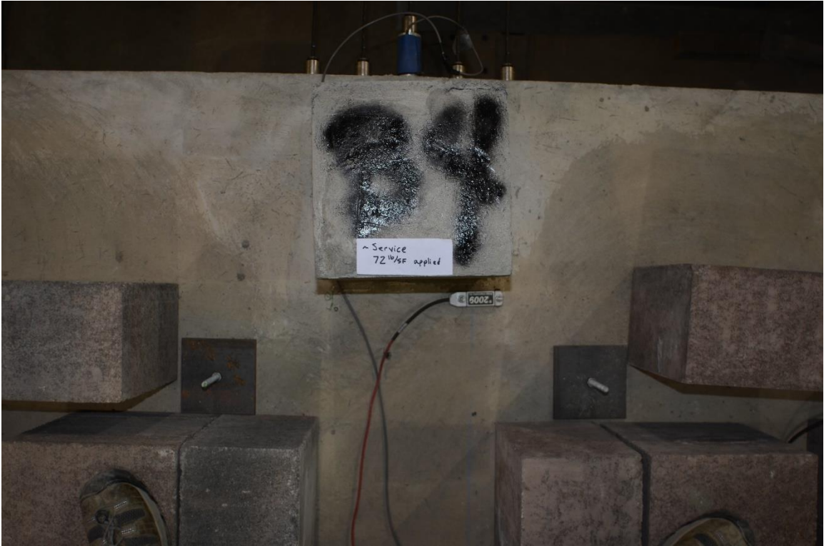
Figure H.31. Column B4 at Service-Level Loading
