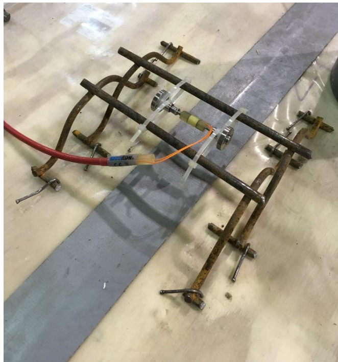
Figure 21. Vibrating Wire Gauge Assembly
