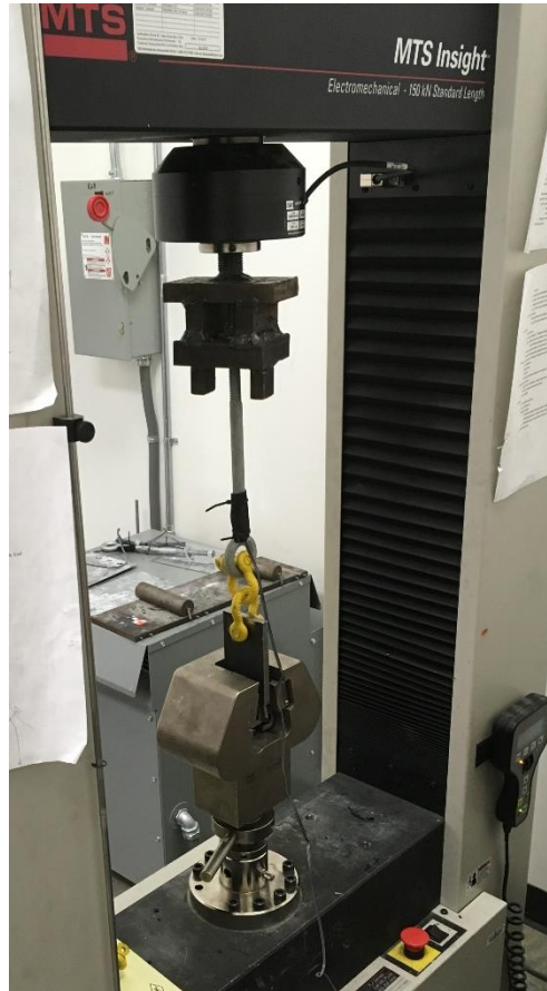
Figure 12. Eyebolt Calibration Setup
