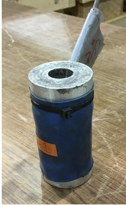
Figure 30. Load Cell for Stressing Operation
