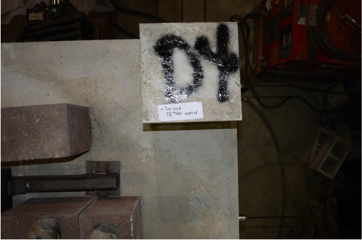
Figure H.29. Column D4 at Service-Level Loading
