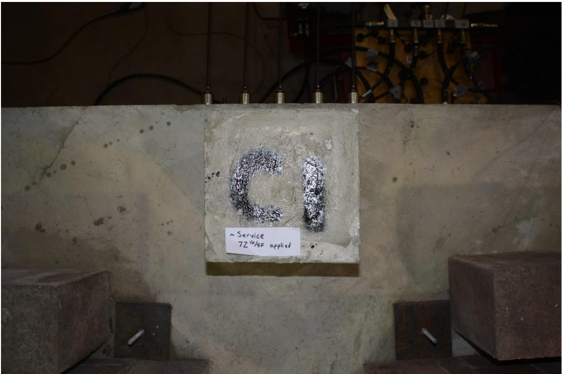
Figure H.18. Column C1 at Service-Level Loading
