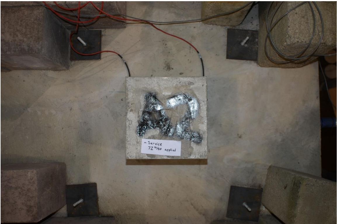
Figure H.24. Column A2 at Service-Level Loading
