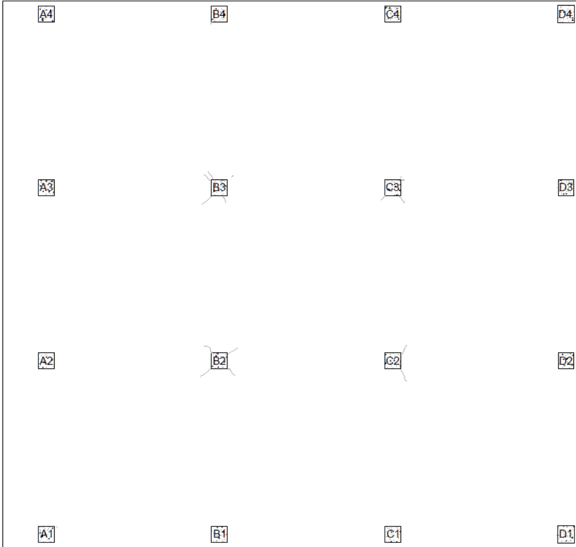
Figure 60. Crack Map at Service-Level Loads
