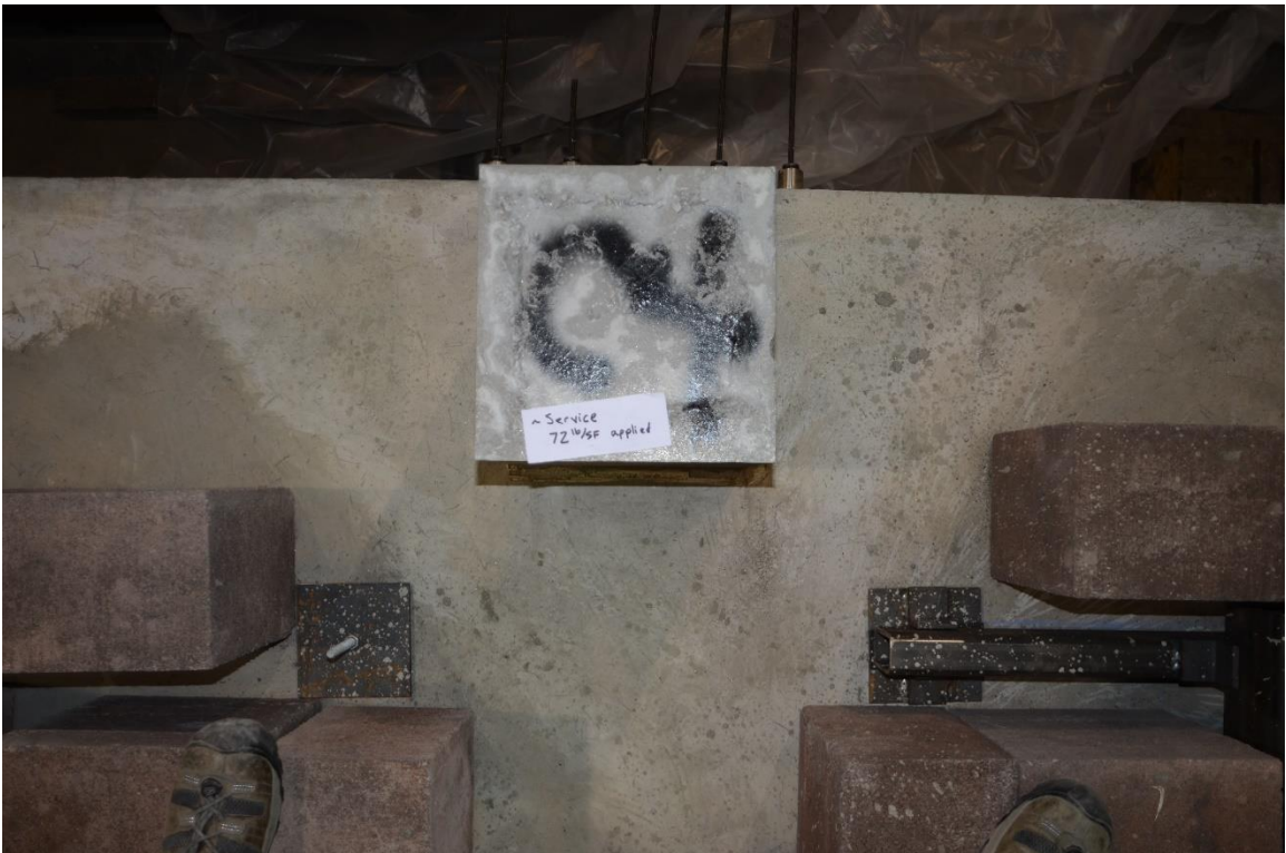
Figure H.30. Column C4 at Service-Level Loading
