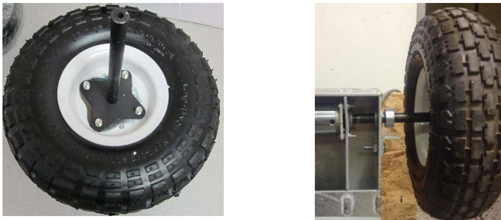
Figure 2-3 the pneumatic tire and the wheel shaft
