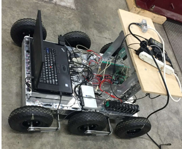
Figure 2-1 the robot chassis with direct drive motors
