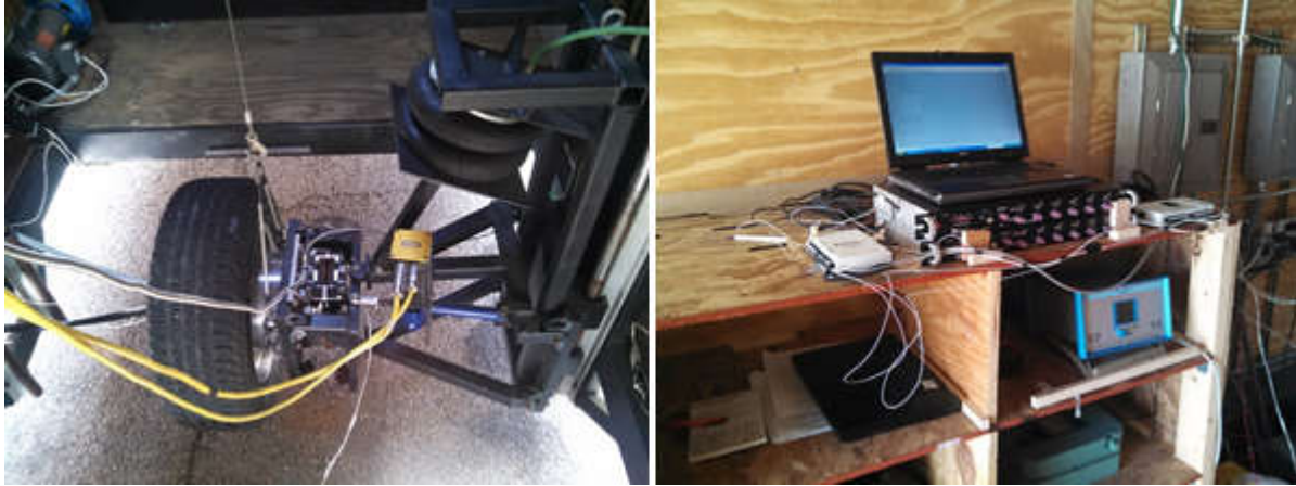
Figure 2-13 quarter car test rig embedded into portable trailer
