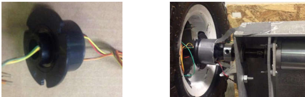
Figure 2-4– Slip ring with six circuit
