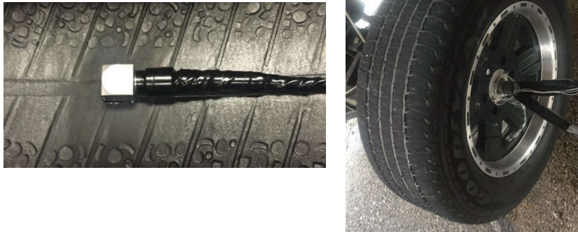
Figure 2-17 tire with a tri-axial accelerometer embedded to its inner liner
