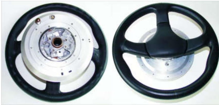
Figure 2-19 the DATRON MSW used in Jetta
