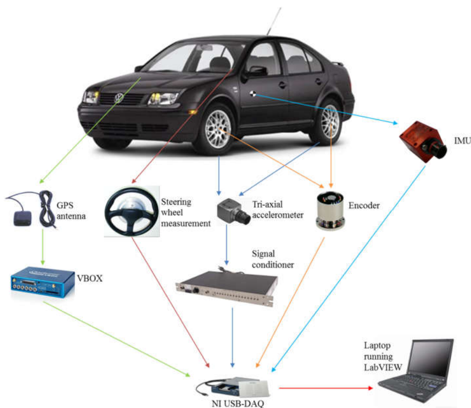
Figure 2-21 the schematic of Jetta's data acquisition System
