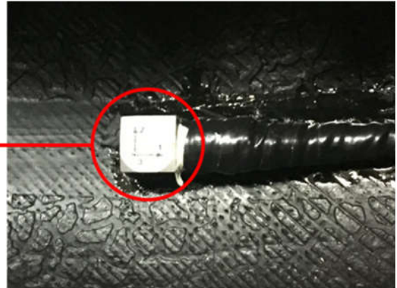
Figure 2-5 Dytran 3023A5 accelerometer attached to the tire
