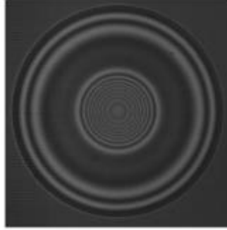
Figure 1-13. Light interference fringes showing droplet deformation. The figure is reproduced from Reference [18] with permission from APS.
