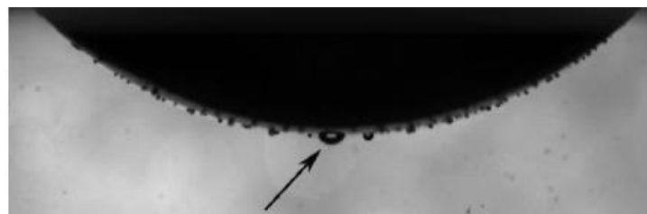
Figure 1-4. Air bubbles observed when a water droplet impacts into water pool simultaneously from side view and bottom view. The droplet diameter is about 3.0mm and the largest air bubble diameter is about 50 \mu m. The figure is reproduced from Reference [55] with permission from CUP.
