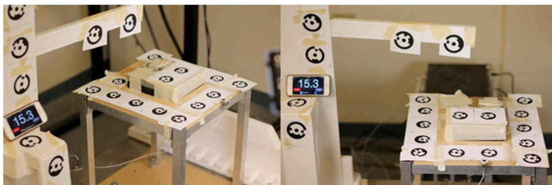
Figure 3. Location of stationary and dynamic coded targets in two synchronized pictures.
