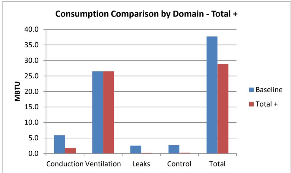
Fig 31. Comparison of energy consumption of retrofit scenario “Total +” and baseline scenario by consumption domain
