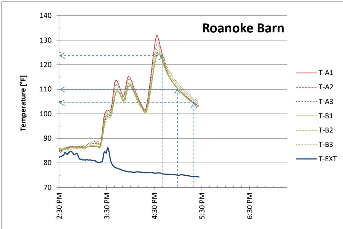
Fig 17. Heat load profile of non-insulated older barn, showing initial furnace issues before running up to the set point temperature.
