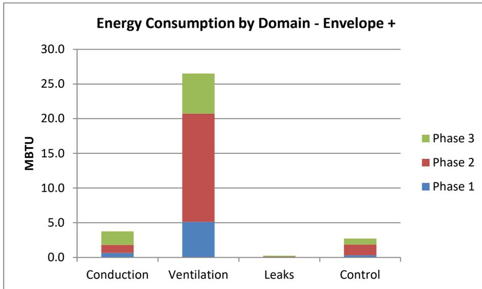
Fig 23. Total energy consumption after retrofit scenario “Envelope +” has been applied. Infiltration leaks can practically be eliminated and conduction losses can be reduced
