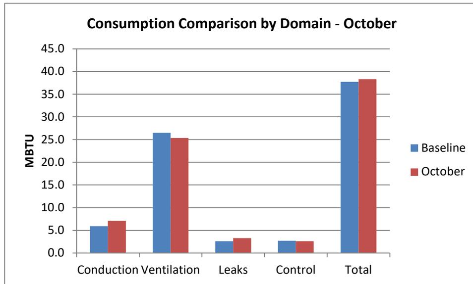
Fig 33. Differences of energy consumption of a curing scenario in October as compared to the baseline scenario under average August conditions
