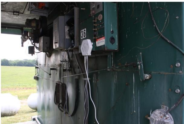
**Fig 14. A second wireless node was used to collect ambient temperature and humidity conditions**
