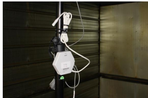
Fig 12. The central sensor recorded temperature and relative humidity, top and bottom sensors were temperature only.
