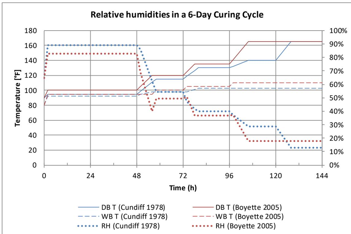
Fig 20. Resulting relative humidity levels over the various curing cycles calculated from dry-bulb and wet-bulb temperature schedules as provided by different sources.
