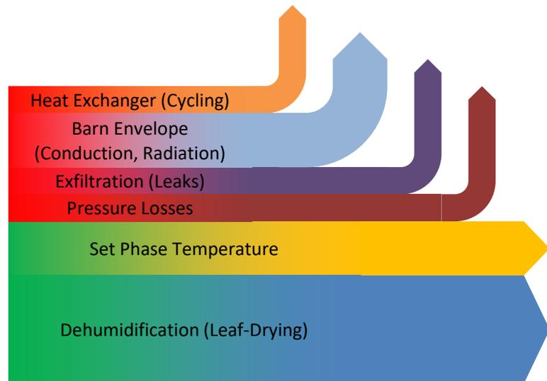
Fig 9. Breakdown of utilization and losses of active processes observed in tobacco curing
