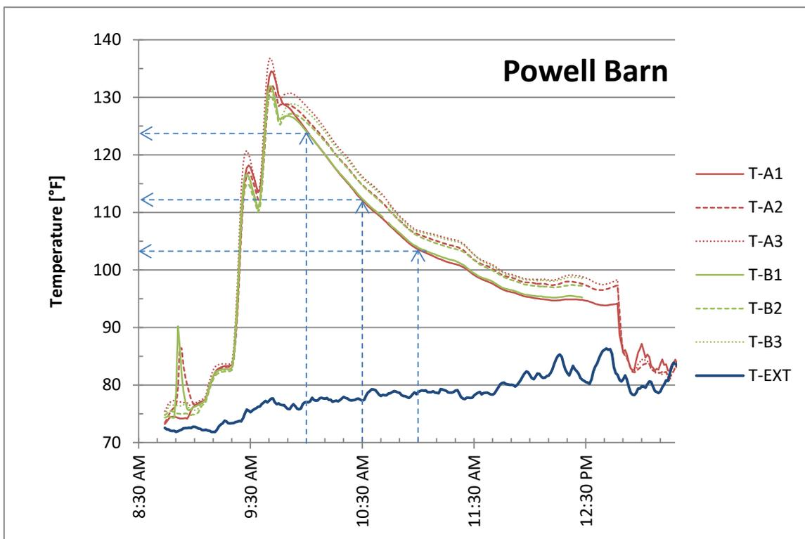
Fig 16. Heat load profile of an insulated newer barn, with initially controlled temperature rise, and subsequent fast rise to set point temperature
