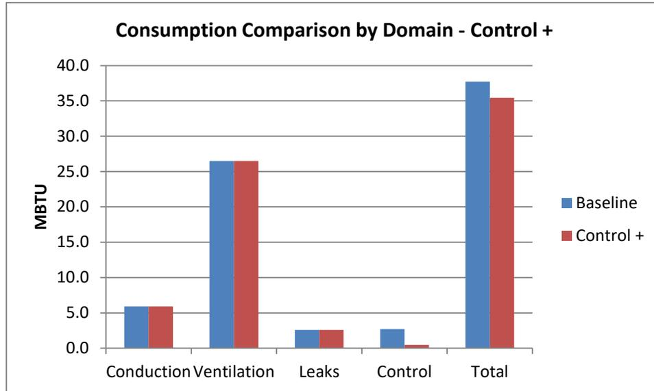
Fig 27. Comparison of energy consumption of retrofit scenario “Control +” and baseline scenario by consumption domain
