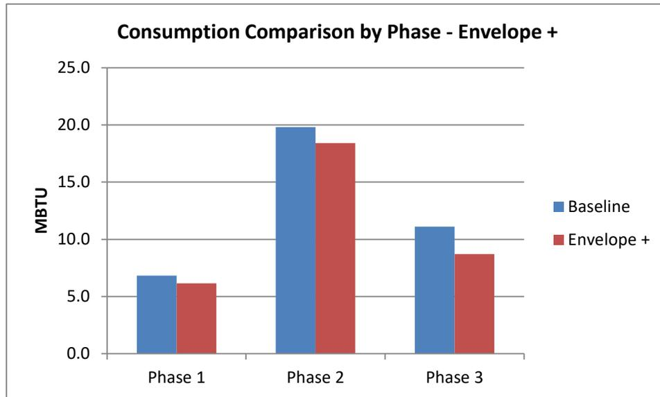
Fig 25. Comparison of energy consumption of retrofit scenario “Envelope +” and baseline scenario by curing phase
