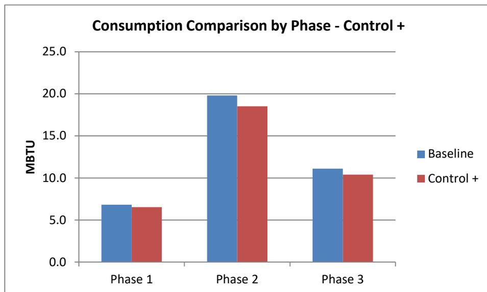
Fig 28. Comparison of energy consumption of retrofit scenario “Control +” and baseline scenario by curing phase
