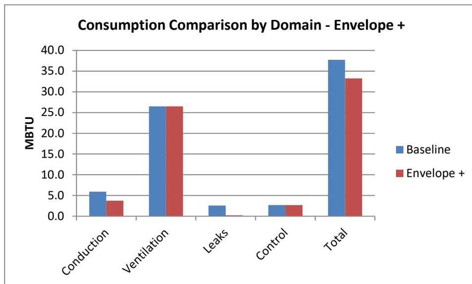
Fig 24. Comparison of energy consumption of retrofit scenario “Envelope +” and baseline scenario by consumption domain
