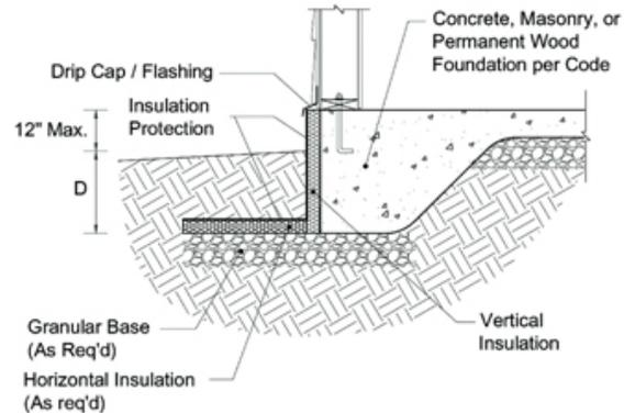
Fig 29. Introduction of a possible additional slab insulation for scenario evaluation purposes
