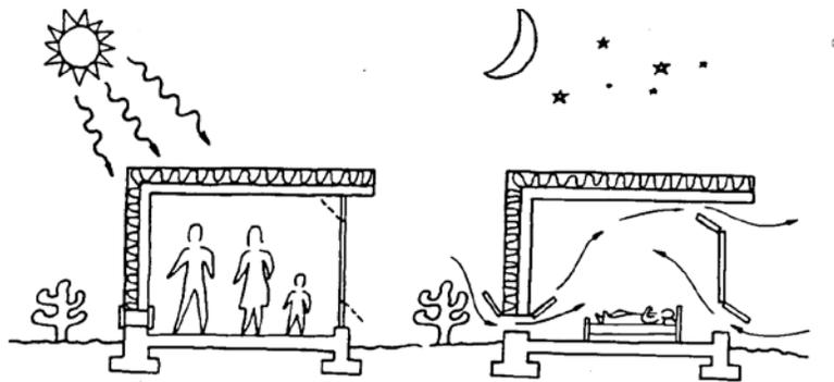
Fig 7. Solar radiation versus night sky radiation needs to be evaluated when looking into harvesting solar energy
