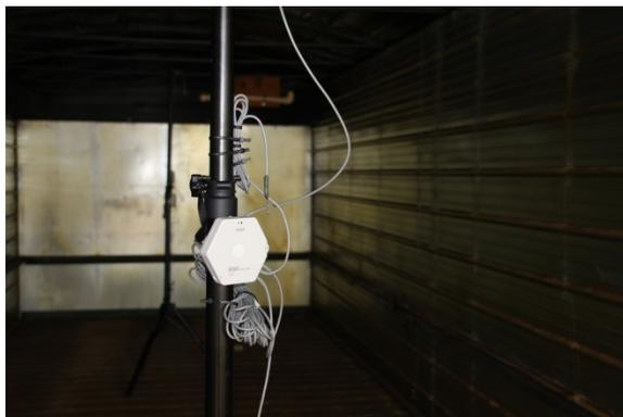
Fig 11. Two poles with temperature probes were placed within the curing compartment of the empty barn
