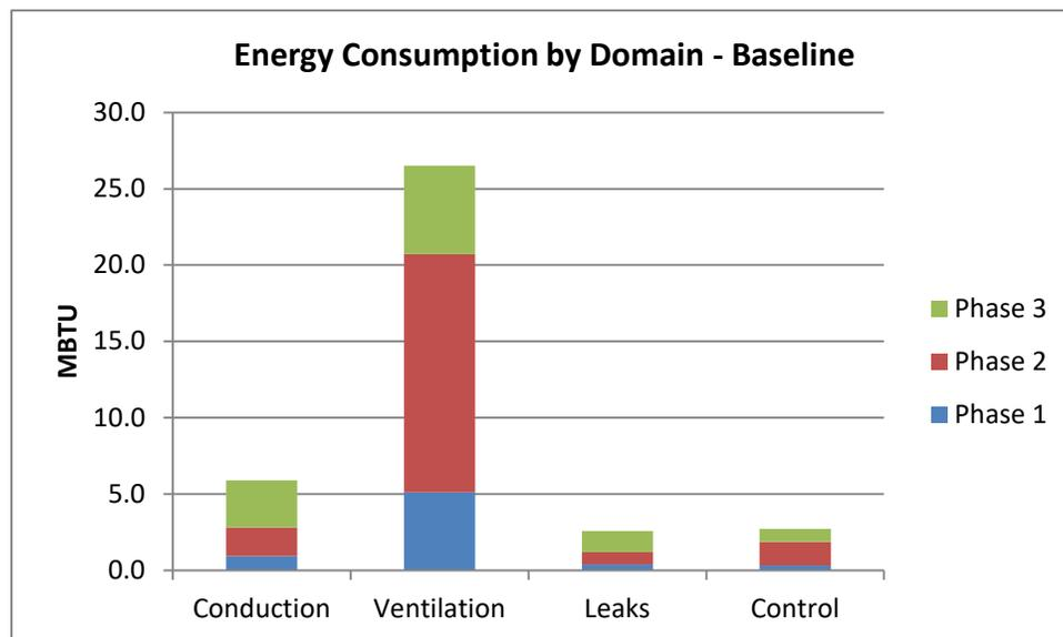
Fig 21. Total energy consumption of tobacco curing broken down by consumption domains.
