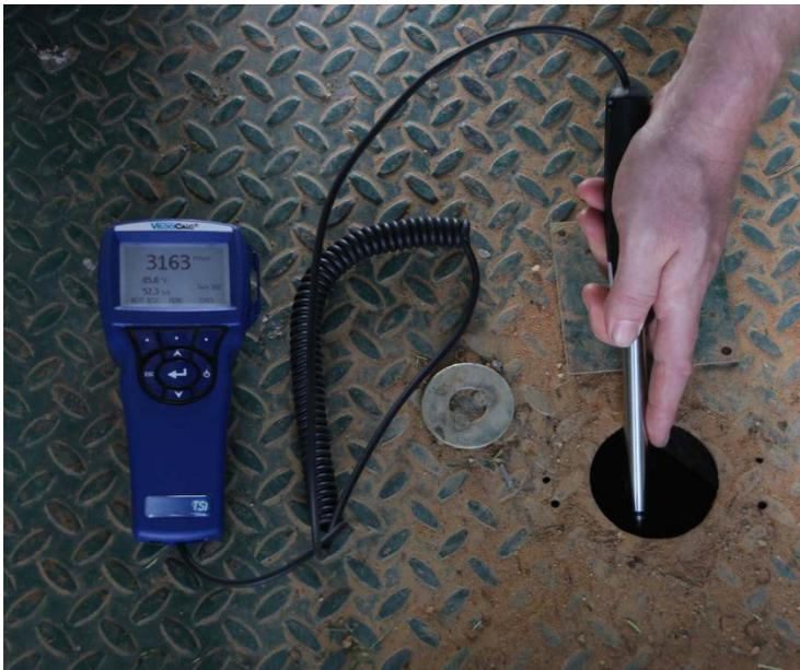
Fig 18. Central velocity in supply plenum between heat exchanger and curing compartment
