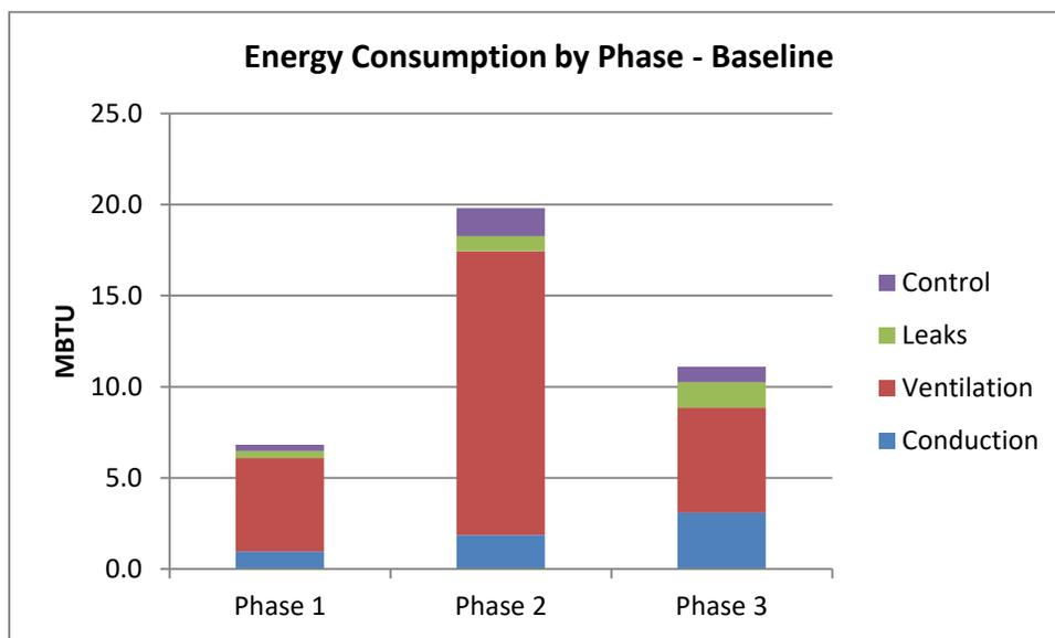
Fig 22. Total energy consumption of tobacco curing broken down by curing phases. Phase 1 – Yellowing, Phase 2 – Leaf Drying, Phase 3 – Stem Drying
