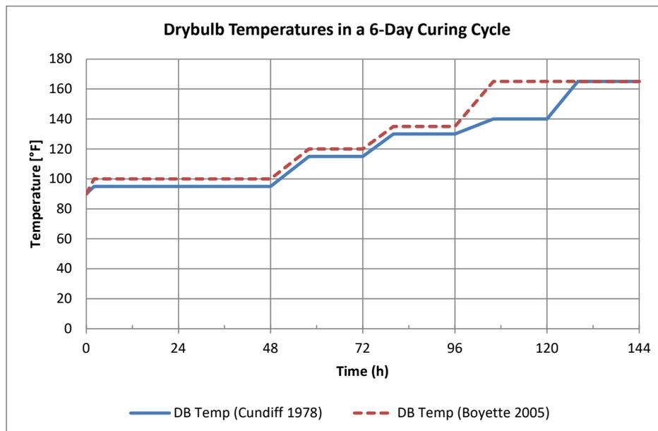
Fig 10. Drybulb temperatures in curing cycles according to different sources
