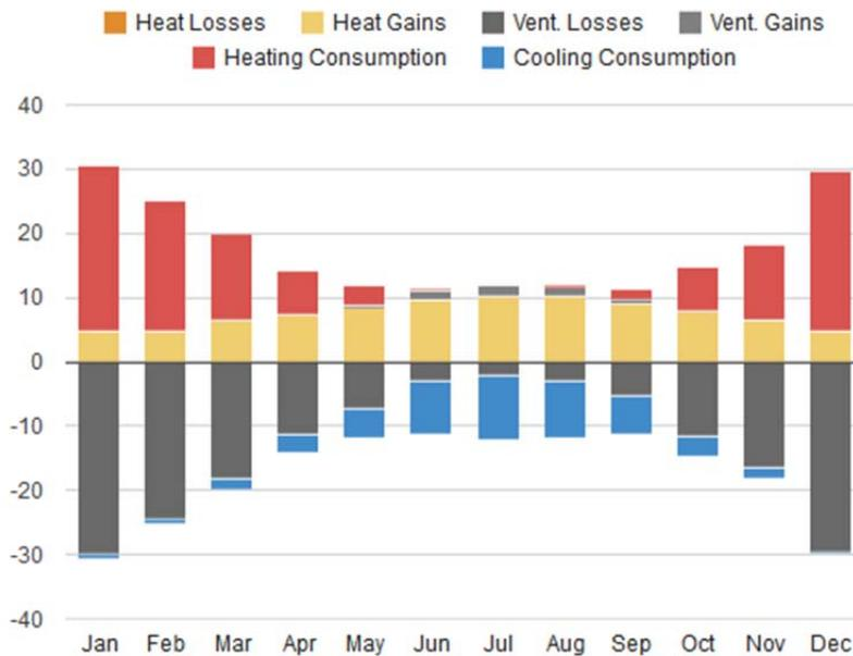
Fig. 15 Derrig 5065 Baseline – monthly loads and consumptions for heating/cooling.
