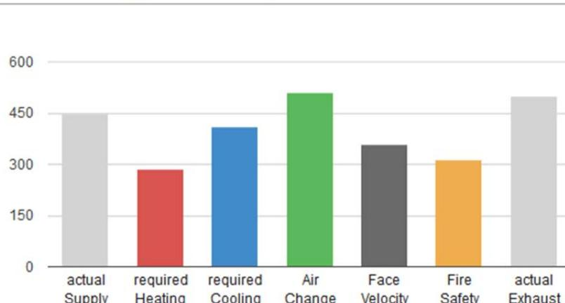
Fig. 17 Derring 5065 Retrofit Scenario – Volume requirements from design mandates
