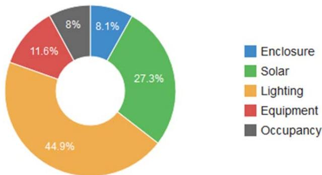
Fig. 6 Derring 5061 Baseline – Cooling loads by heat gains sources.
