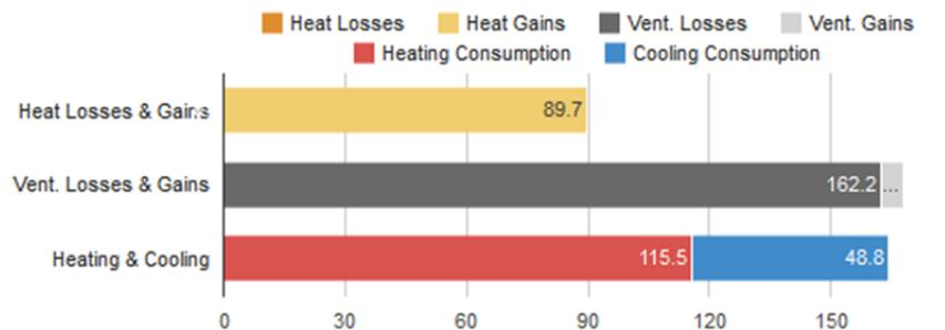
Fig. 16 Derrig 5065 Baseline – Annual comparison of energy losses, gains, and systems consumption to meet heating and cooling demands.
