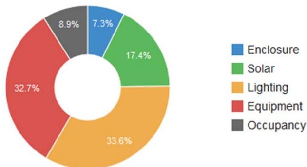
Fig. 14 Derring 5065 Baseline – Cooling load requirements by heat gains sources.
