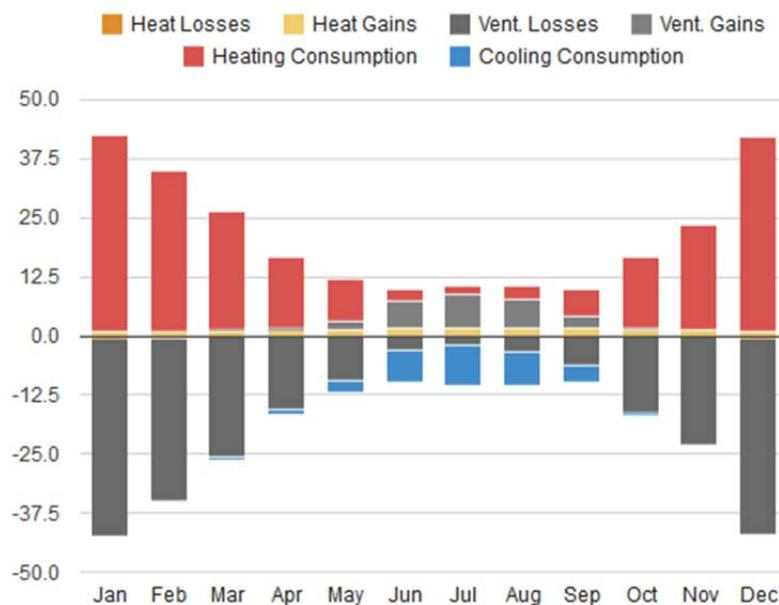
Fig. 7 Derring 5061 Baseline – monthly energy losses, gains, and consumption balances.
