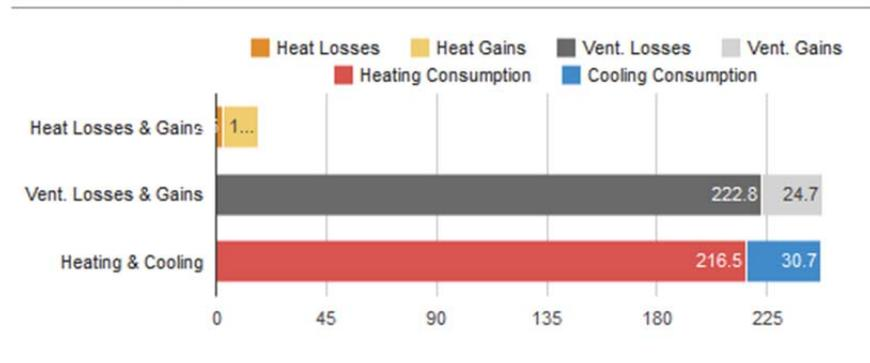
Fig. 8 Derring 5061 Baseline - Comparison of annual heating gains/losses, ventilation gains/losses and resulting heating/cooling energy consumption.
