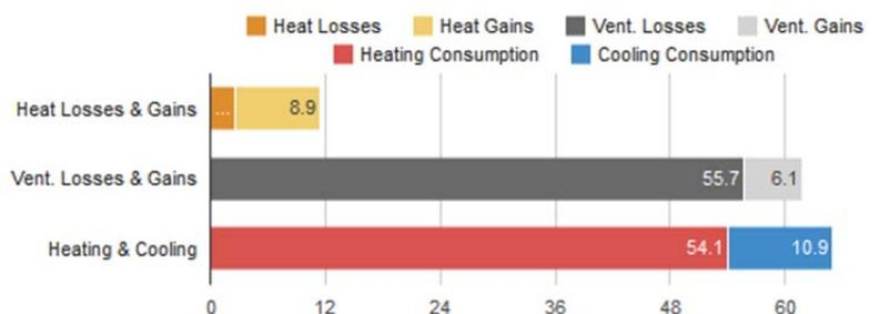
Fig. 12 Derrig 5061 Scenario 2 – Monthly and annual energy balances after installation of retrofit kits into both fume hoods coupled with other performance improvements for the laboratory space.
