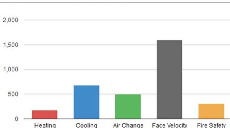
Fig. 5 Derring 5061 Baseline – Volume requirements to meet design mandates.
