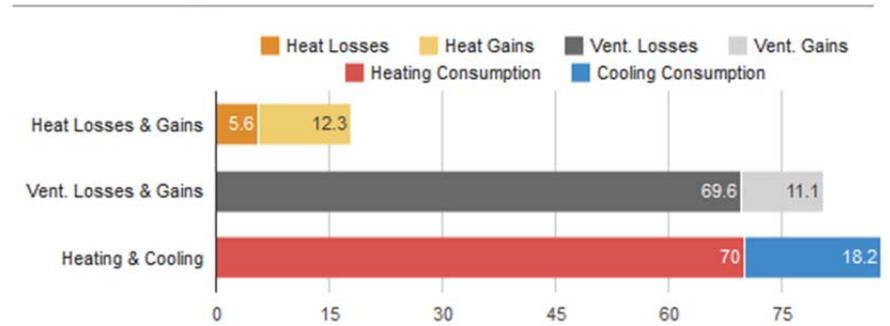
Fig. 18 Derring 5065 Retrofit Scenario – Energy balances from loads and ventilation, and required heating/cooling consumptions – New Fume Hood Lab Space.
