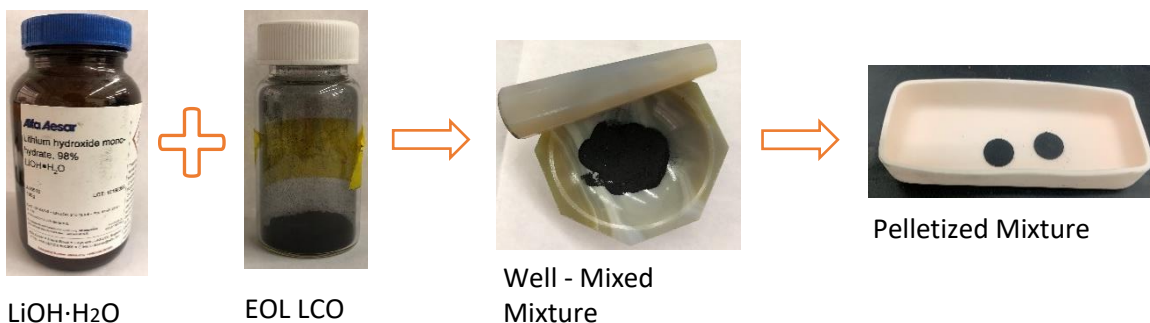
Figure 40. Process of preparing samples for sintering
