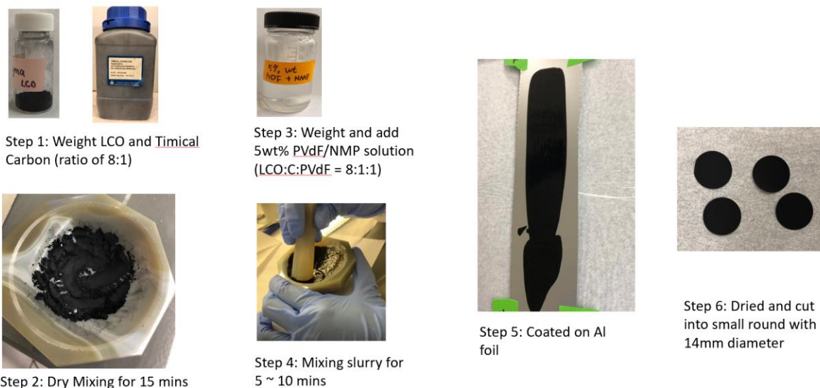
Figure 41. Process of slurry and electrodes preparation
