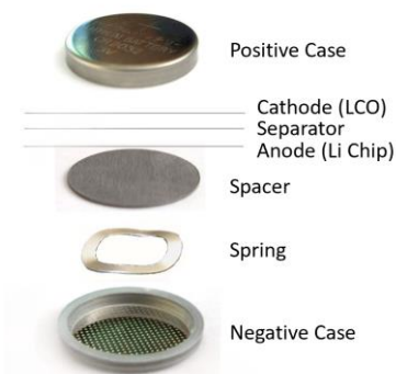
Figure 42. Components of a coin cell
