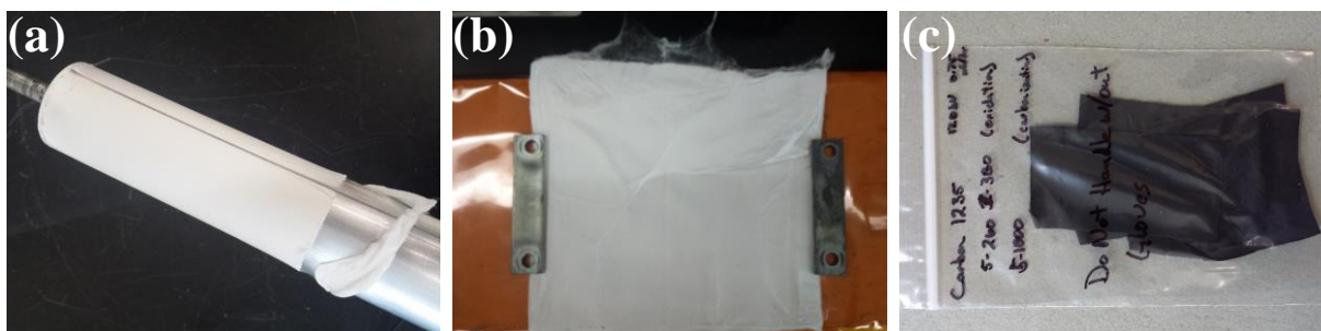
Figure D.14. Electrospun carbon fiber mat prepared from a 12% w/w solution of polyacrylonitrile (PAN) and DMF (a) as prepared, (b) after annealing at 125 °C for 10 minutes, and (c) after oxidation and carbonization.
