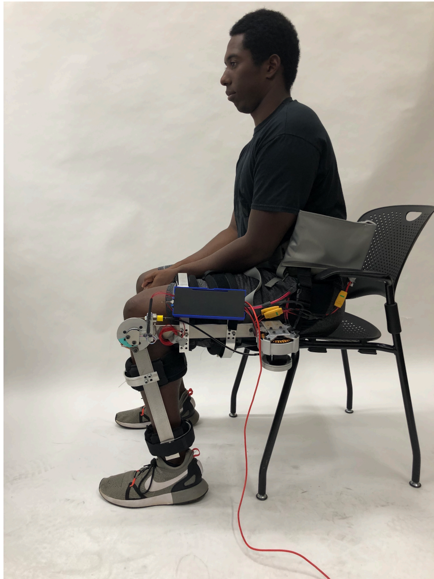
Figure 5.19: Active knee exoskeleton being worn for STS motion testing
