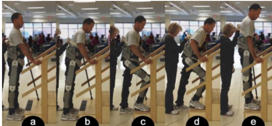
Figure 2.18: Stair negotiation exoskeleton developed at Vanderbilt University to assist paraplegic individuals [14]
