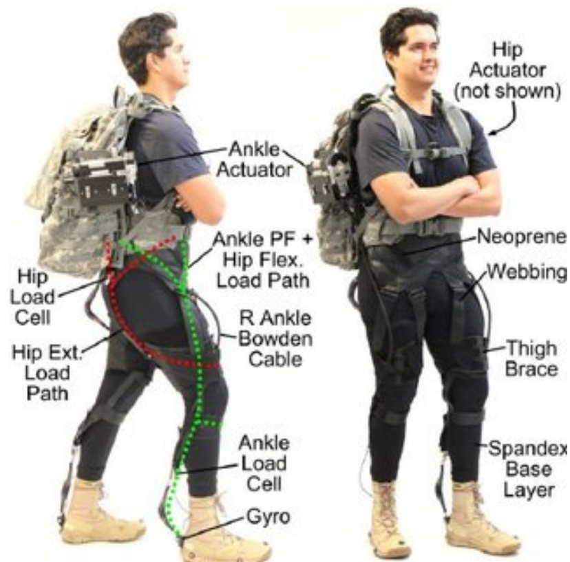
Figure 2.13: Cable driven Exosuit for assistance in walking of up to 4 mph[9]
