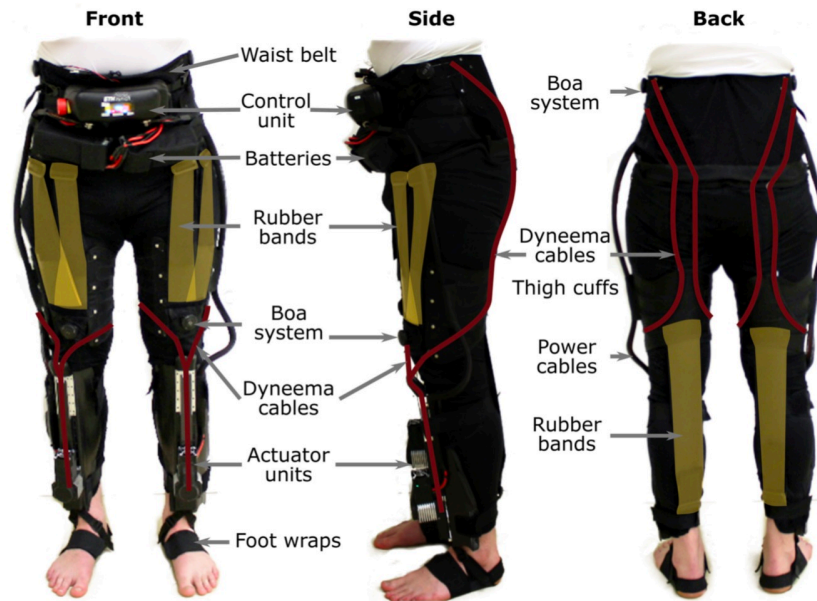
Figure 2.17: Component structure of the Myosuit used to assist individuals suffering from muscle weakness [13]
