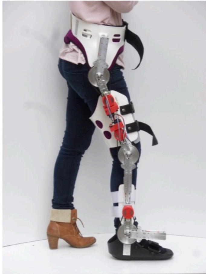
Figure 2.16: STS Exoskeleton using SEA mechanism [12]
