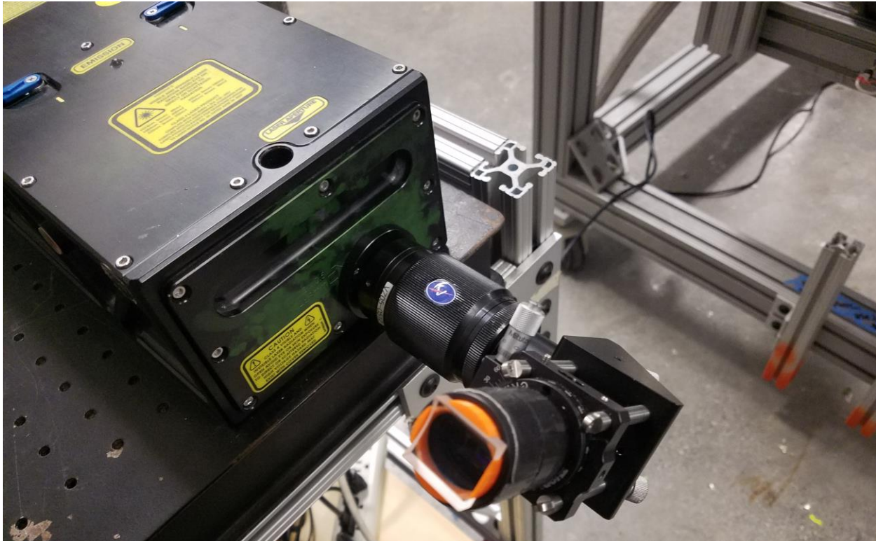
C.2. Quantel Evergreen laser head with mounted collimator, mirror, and cylindrical lenses.
