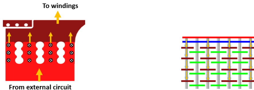
(a) Top view of termination current entering the windings. (b) Front view of termination current entering the windings.
