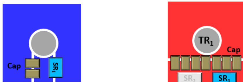
(a) Output capacitors on the old termination design. (b) Output capacitors on the new termination design.
