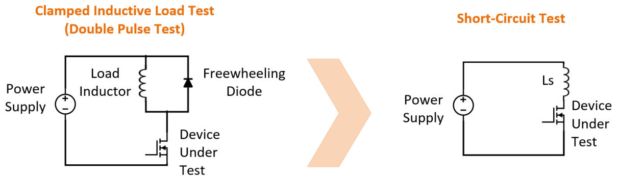
Fig. 27: Schematic showing the differences between the double pulse test and the short-circuit test circuits
