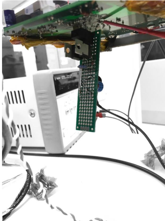
Fig. 70: Attachment of the dynamic-on resistance board for measurement
