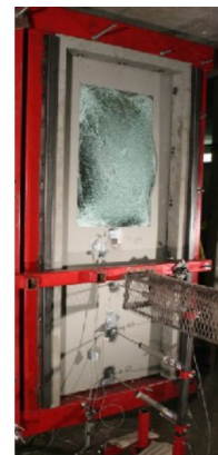
(d) Comparison of small and large window failures
