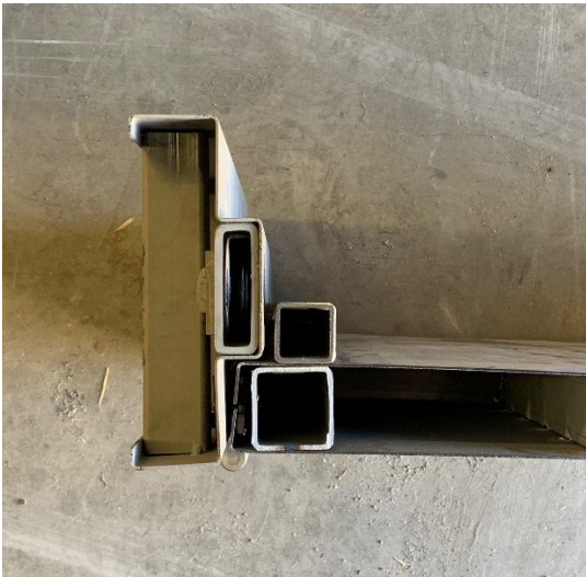
(c) Test 5A frame-skin deformation.
