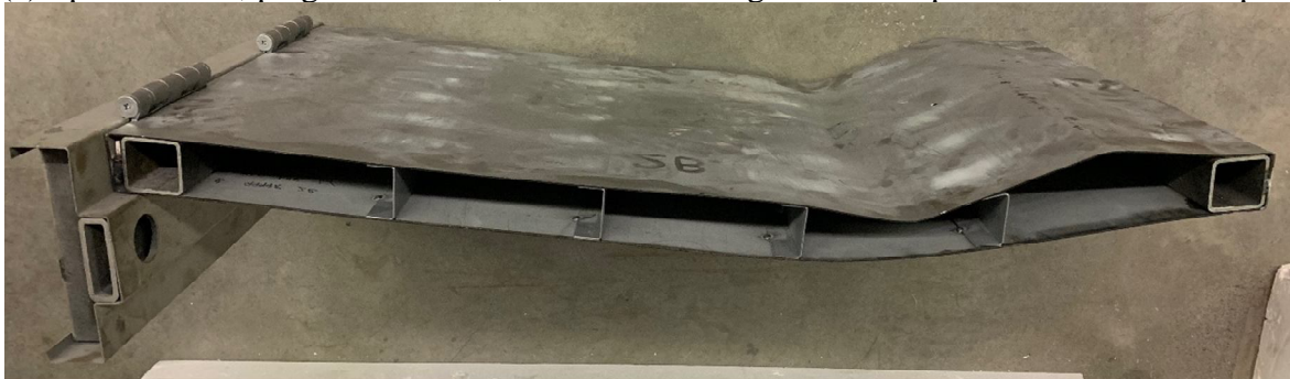
(b) Specimen 2B, plug weld failure, and skin buckling in the shear span on the latch side.
