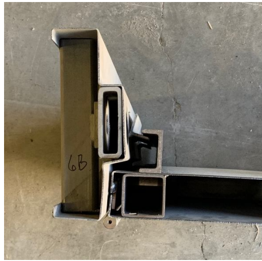
(b) Test 6B frame-skin deformation.
