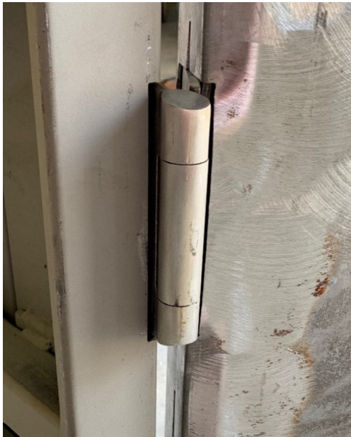
(c) Series 9A deformed hinge plates from bottom of the specimen.
