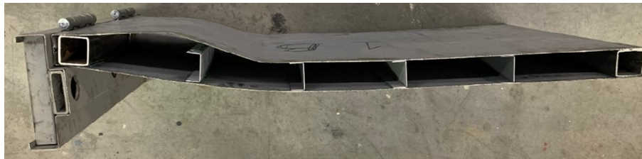
(b) Specimen 1B, epoxy failure on hinge side.
