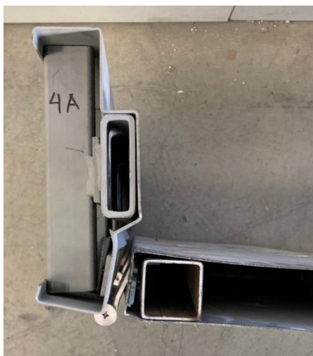
(a) Test 4A skin deformation.
