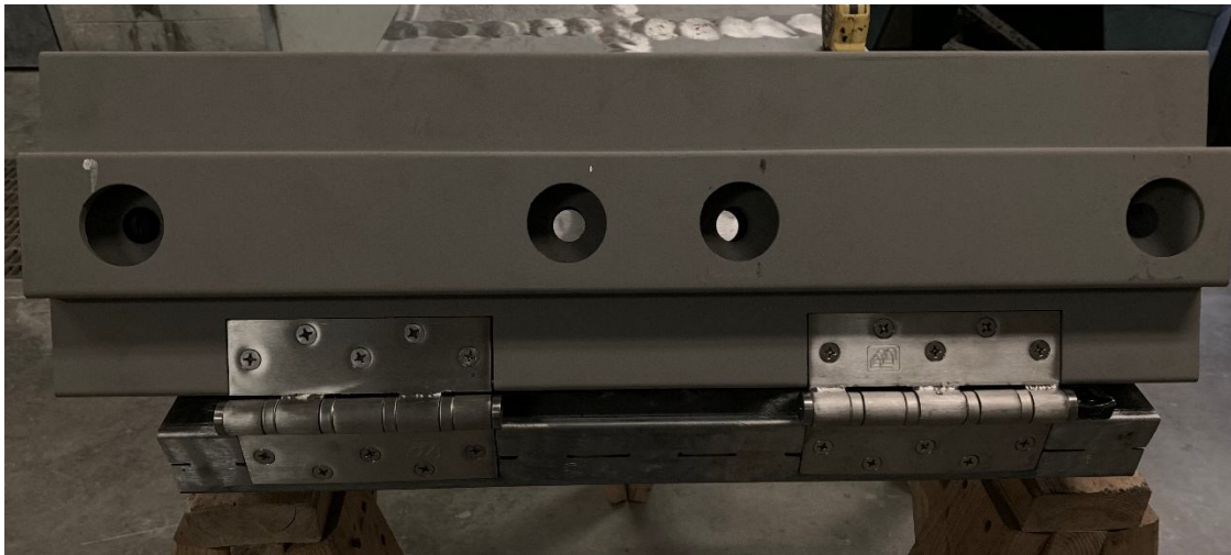
Figure 2.3: 6'' PBB Stainless Hinges (Series 4).
