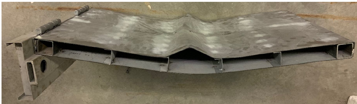
(a) Specimen 3A, plug weld failure, and skin buckling on the compression skin at mid-span.
