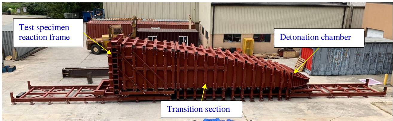
Figure A.2: Photograph of Virginia Tech Shock Tube Testing Facility.
