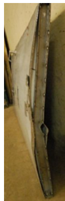
(b) Failure along the bottom of the rigid insulation specimen
