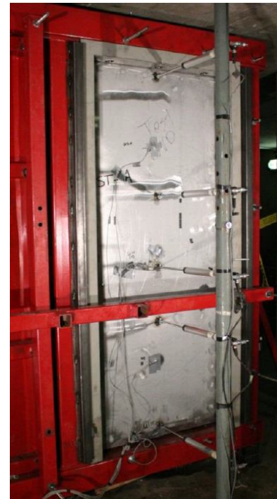
(b) ST-9A door assembly mounted in test fixture.
