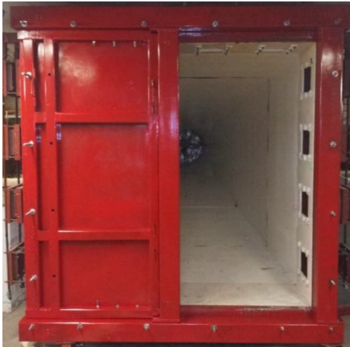
(a) Shock tube test fixture for full-size door assemblies.
