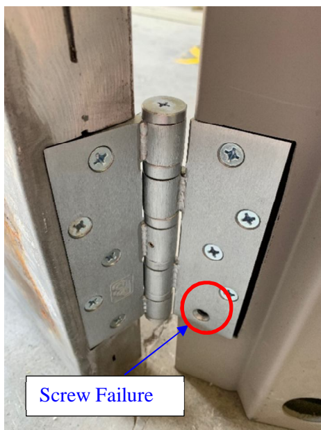
(b) Series 9A deformed hinge plates and deformation in door-skin.
