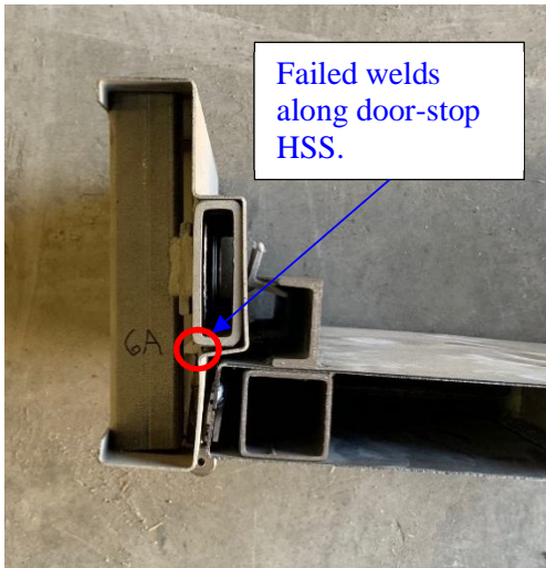
(a) Test 6A frame-skin deformation.
