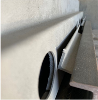
(a) Retainer angle weld failure and deformation (from test 6A).
