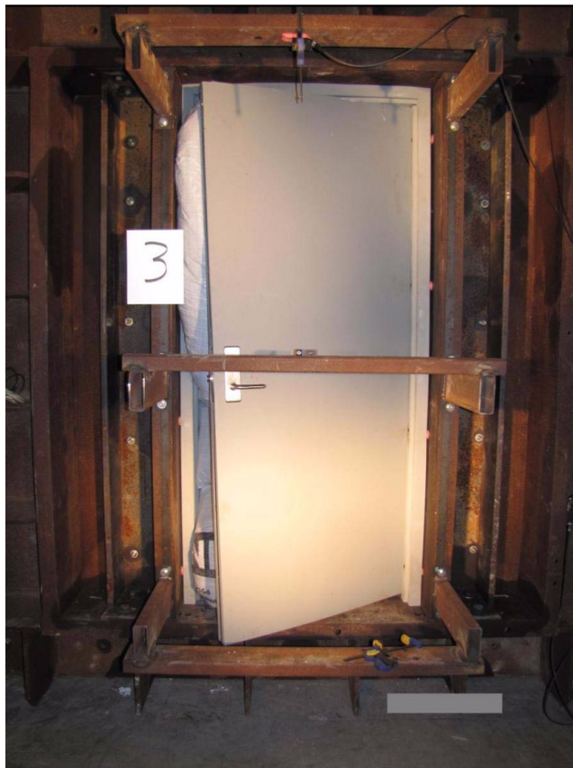
(a) Door assembly after dynamic testing.
