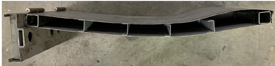
(a) Specimen 1A, epoxy failure on latch side.
