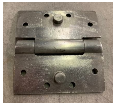
(c) Mortise pin which interlocks with frame and door hinge mount plates.
