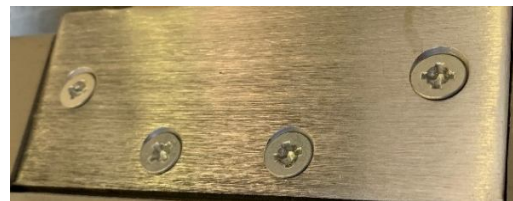
(b) Typical hinge leaf slip observed.
