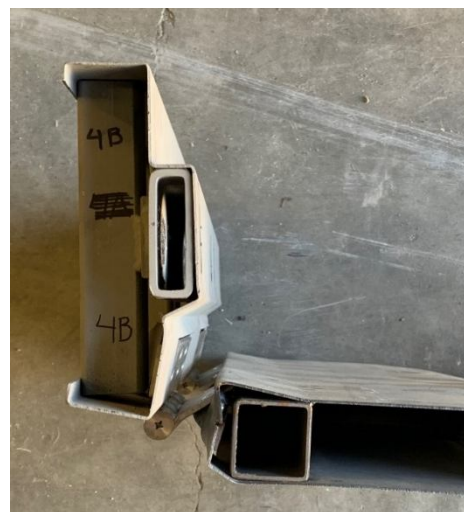
(b) Test 4B skin deformation.
