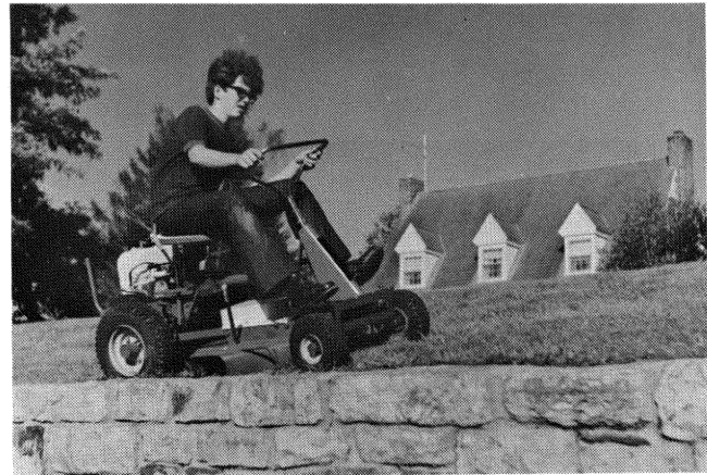
Figure 12. Too much speed near ditches and retaining walls can be dangerous.
