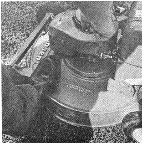
Figure 6. When starting engine, mower may be steadied by placing foot in a safe position on machine.
