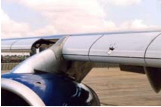
(a) Damage observed at leading edge
