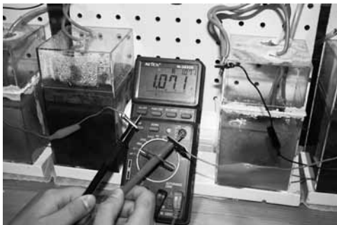
Microbial Fuel Cell – Voltage Reading (MFCs in series circuit)
