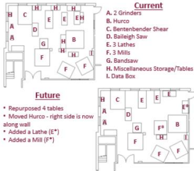
FIGURE III CURRENT MACHINE SHOP LAYOUT AND FUTURE MACHINE SHOP LAYOUT
