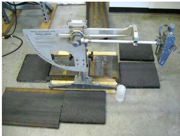
**Figure 2. British Pendulum Tester Testing Asphalt Concrete Slabs**
