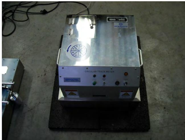
Figure 4. Macrotexture Measurement of Asphalt Concrete Slabs Using the Circular Texture Meter
