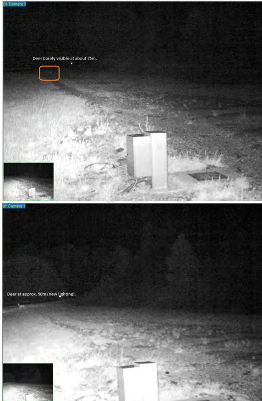
Figure 14. Improved Site Illumination After Installing Additional NIR Illuminators (bottom)
