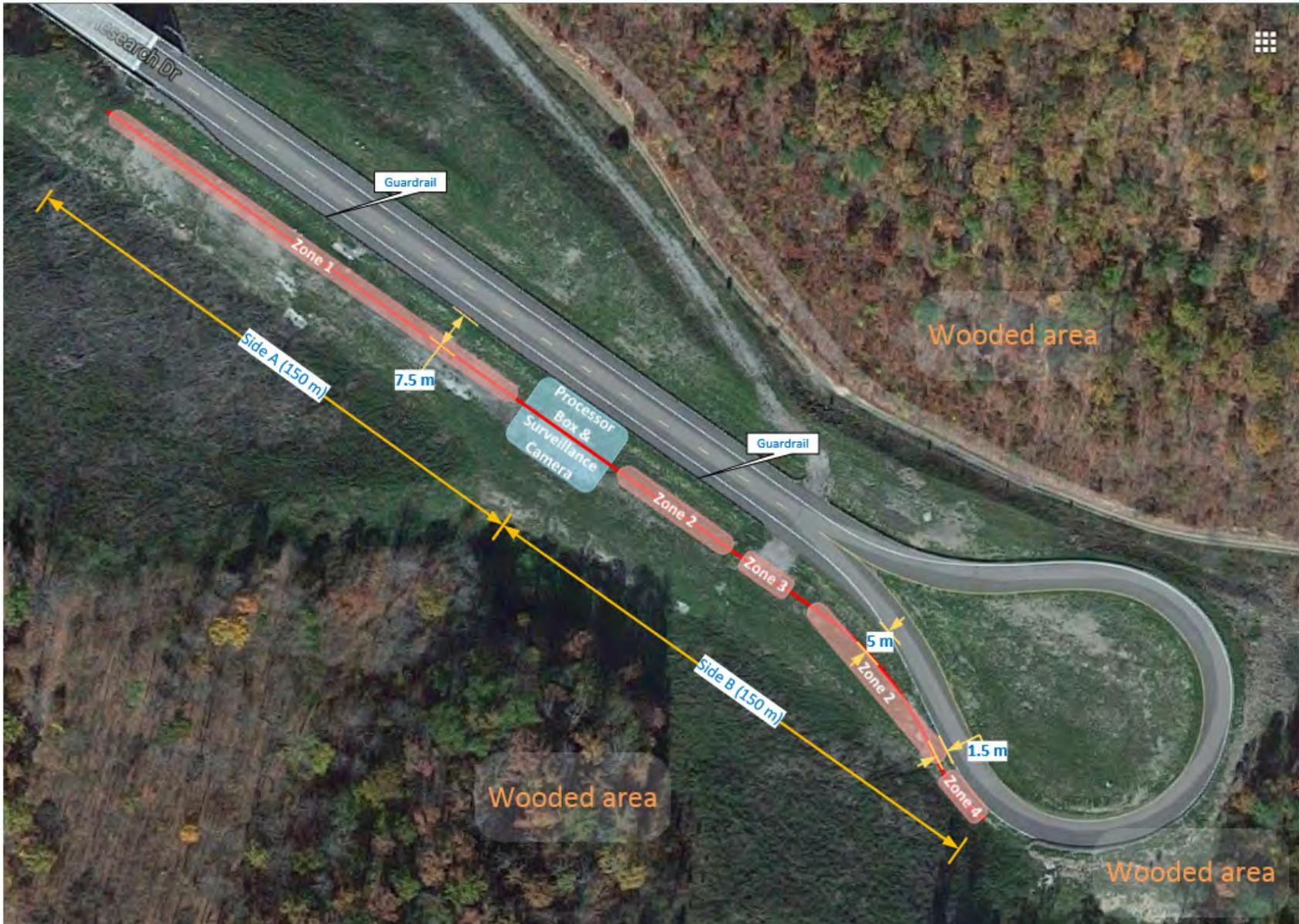
Figure 3. ADS Installation Location and Detection Zones
