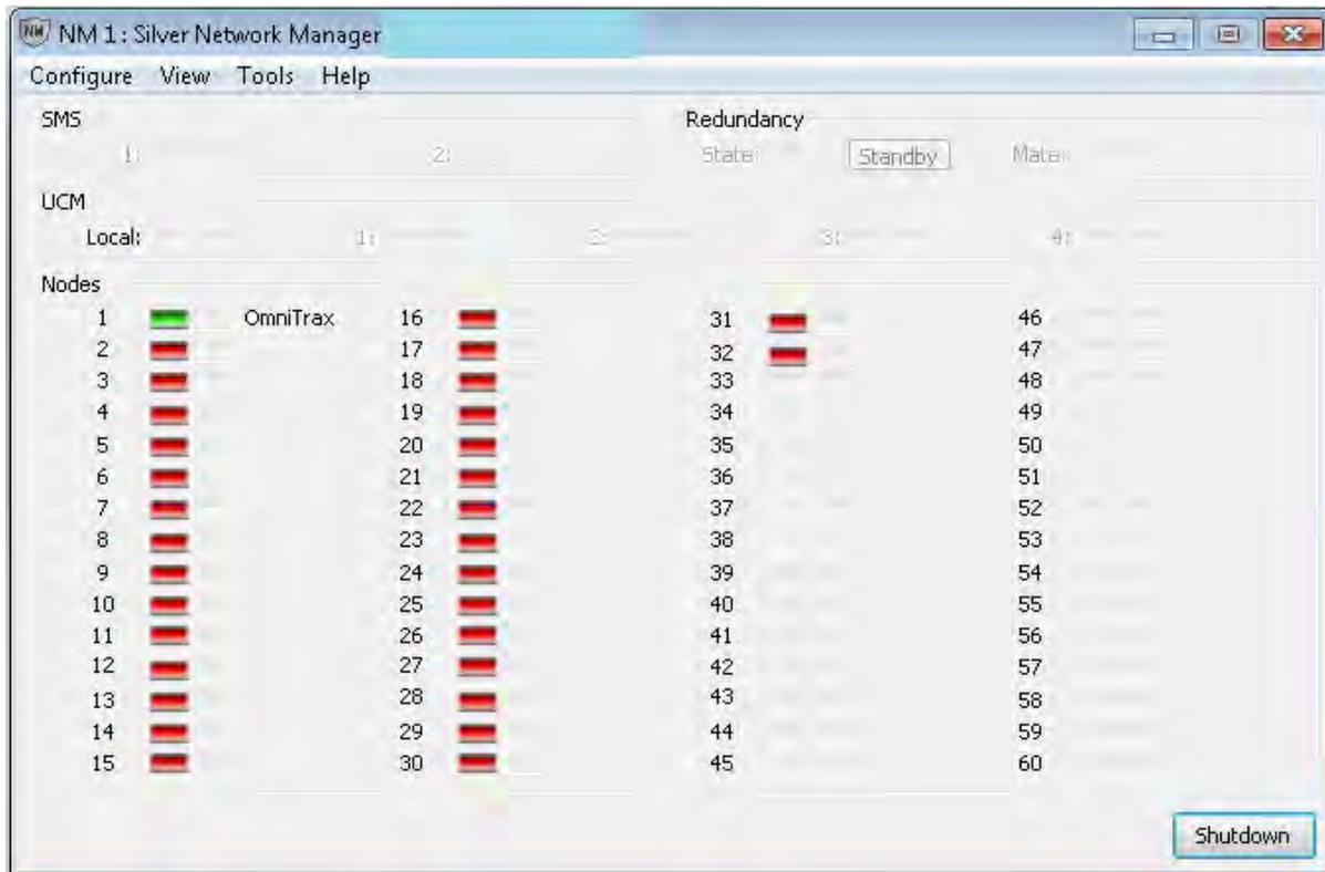
**Figure 10. Network Manager Program That Ensures Communication Between Processor and Data Storage Computer. Communication was established through a single-mode fiber optic cable available on the Smart Road.**
