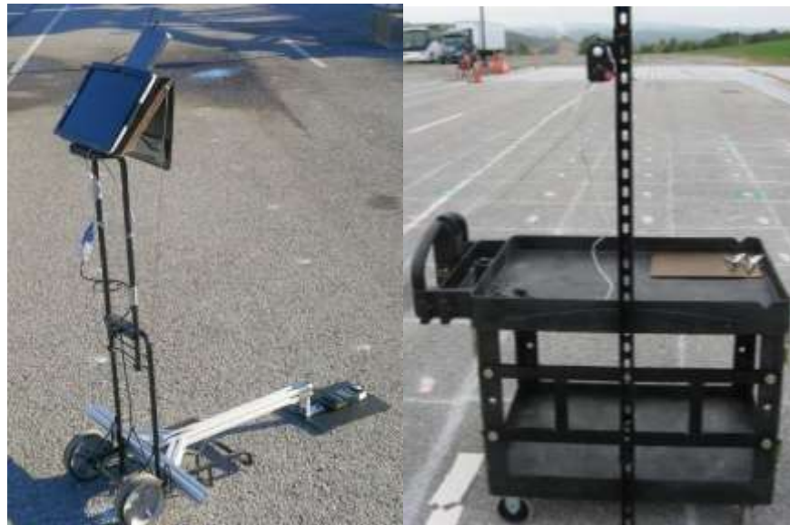
Figure 3. Horizontal and Vertical Illuminance Measurement Systems
