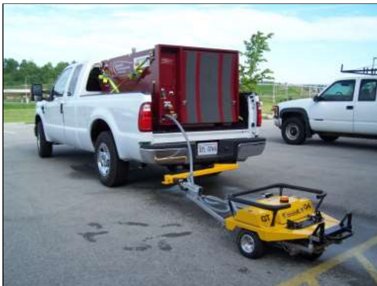
Figure 1. VTTI's Grip Tester, CFME Available in Virginia.
