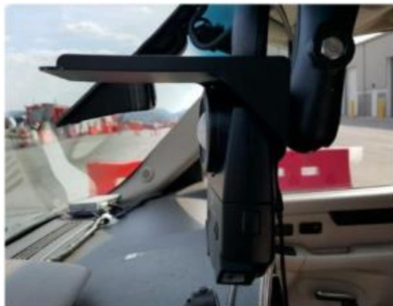
Figure 70. Mounting of the cosine-corrected illuminance meter on windshield to measure vertical illuminance levels.
