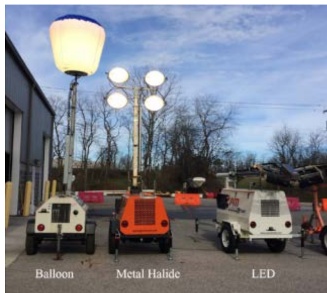
Figure 3. Portable light towers used in Virginia Smart Road characterization.
