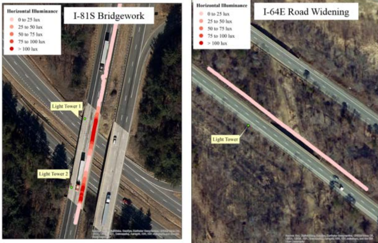
Figure 28. Horizontal illuminance levels at two work zones with differences based on number of lanes and light towers.
