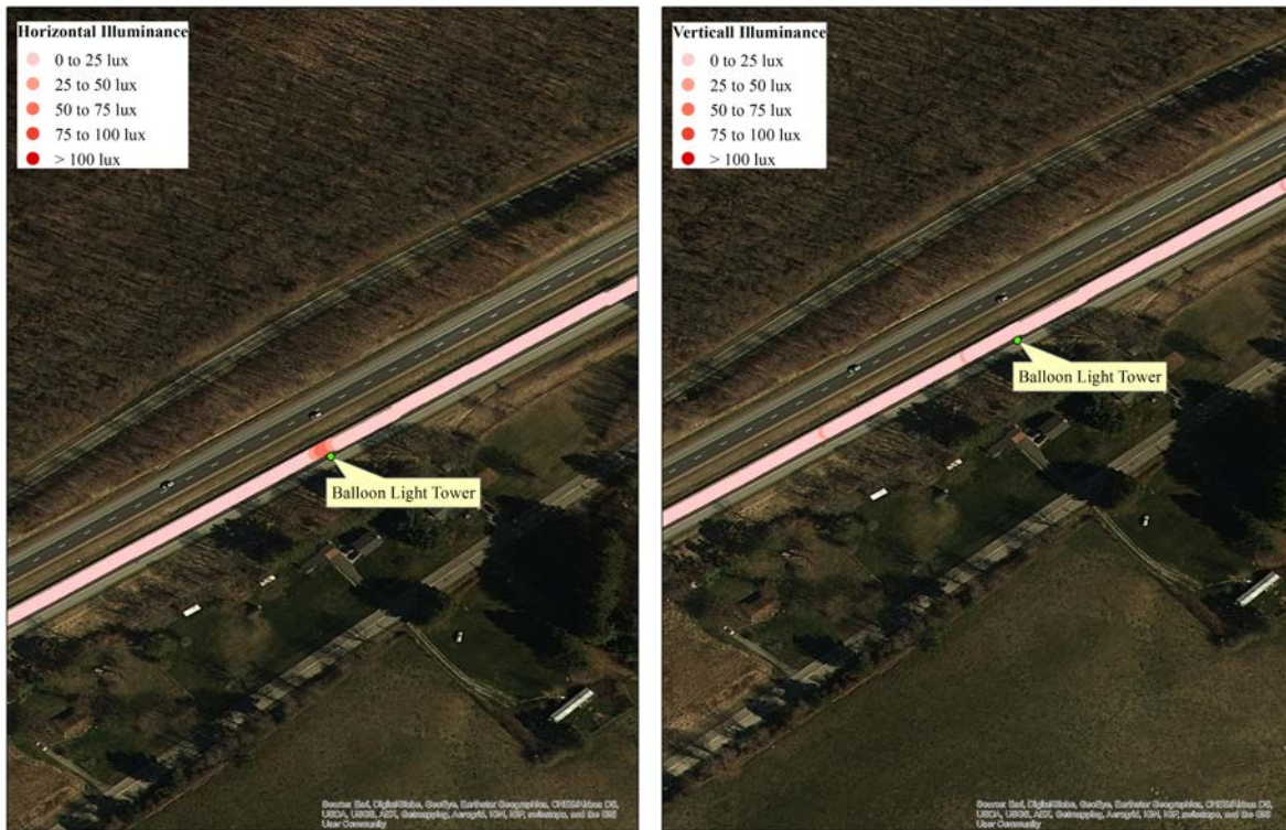
Figure 13. Horizontal and vertical illuminance levels at the milling and paving operation on I-81 north.
