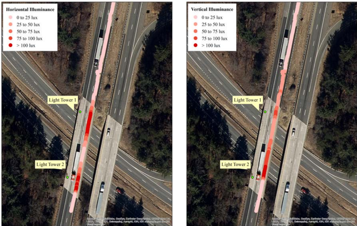
Figure 9. Horizontal and vertical illuminance levels at the I-81 south bridge work.
