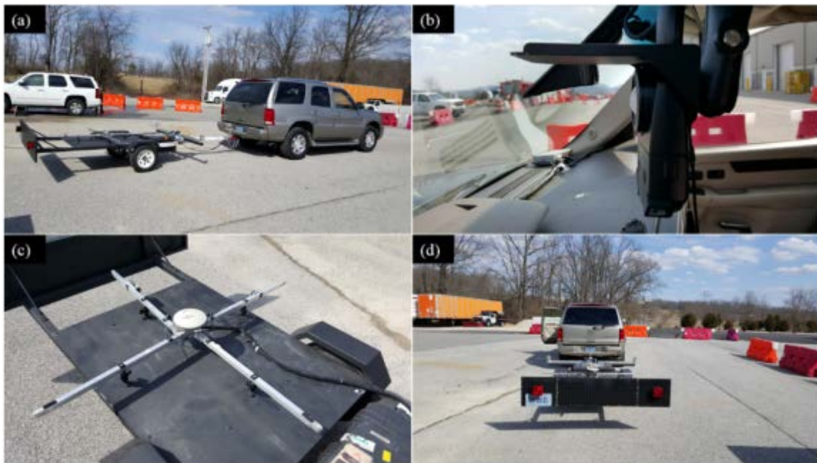
Figure 2. TRLMMS developed at VTTI. (a) TRLMMS hitched to vehicle. (b) Illuminance meter that measures the vertical illuminance mounted to the windshield. (c) “Spider” apparatus with GPS unit in the center. (d) TRLMMS from behind with the headlamp barrier that eliminates the influence of the following vehicle’s headlamps.
