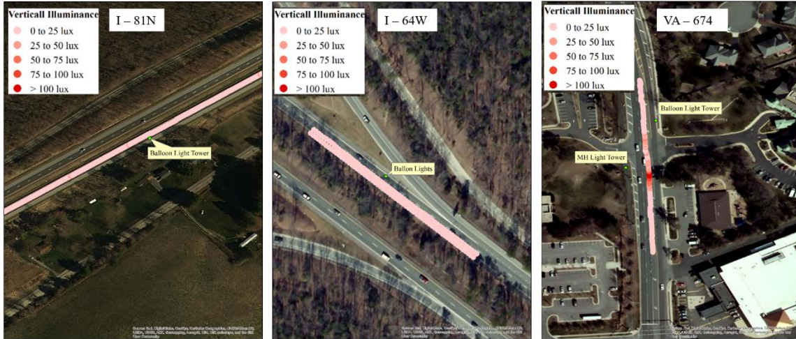
Figure 35. Comparison of vertical illuminance levels in milling and paving operations using equipment-mounted and portable light towers.
