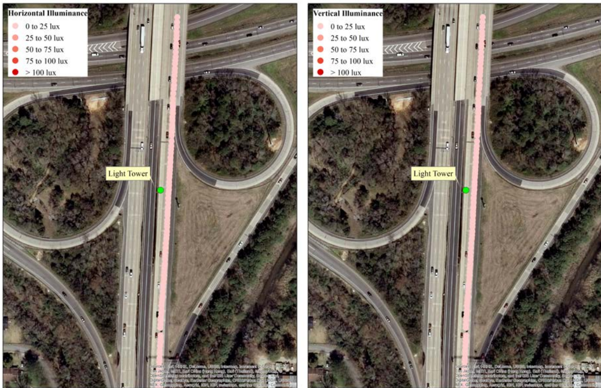
Figure 19. Horizontal and vertical illuminance levels at the trench drain installation on I-64 West.
