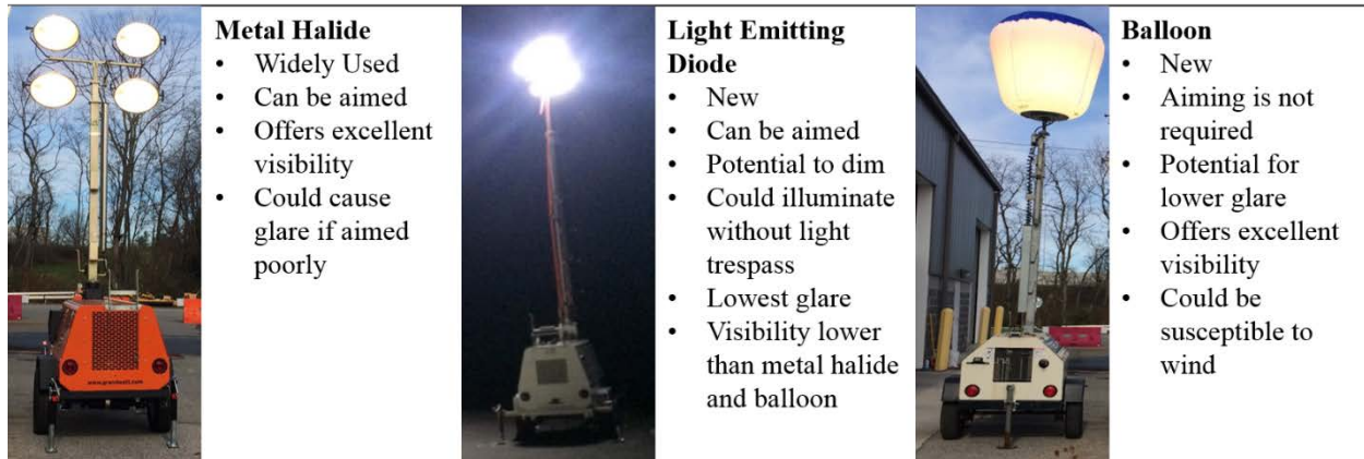
Figure 73. Features of the three light tower types used in the Virginia Smart Road evaluation.
