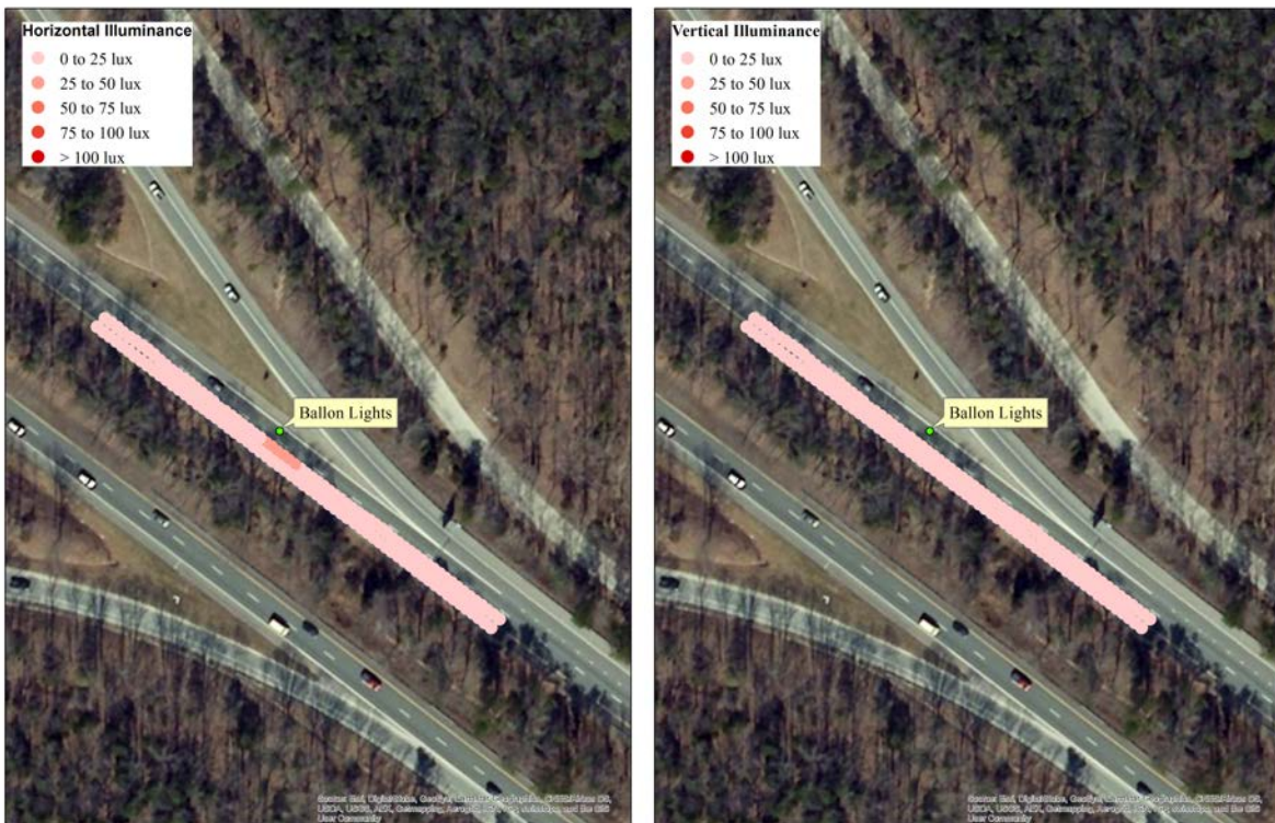
Figure 23. Horizontal and vertical illuminance levels at the milling and paving operation on I-64 west.
