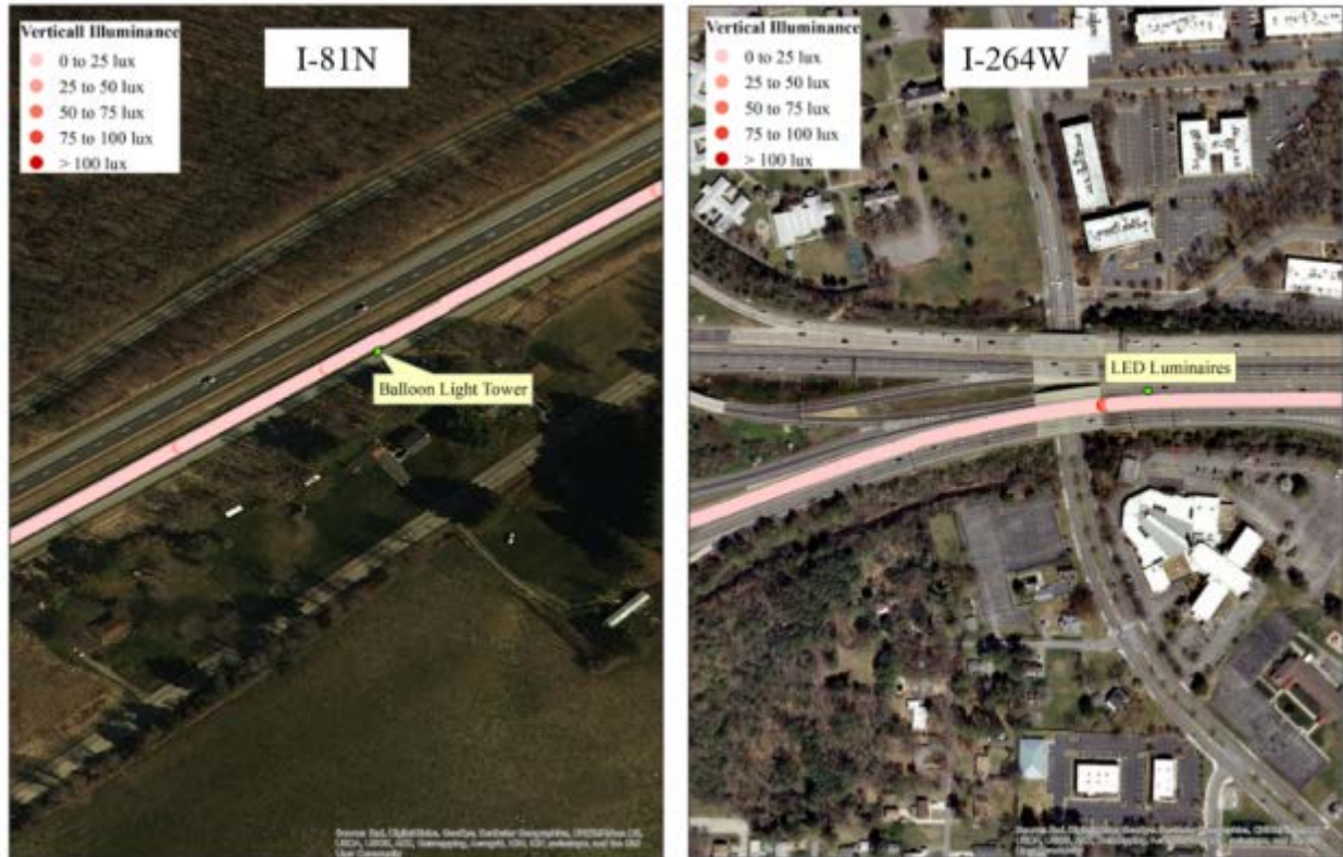
Figure 37. Differences in the distribution of vertical illuminance levels in equipment-mounted balloon vs. LED luminaires.
