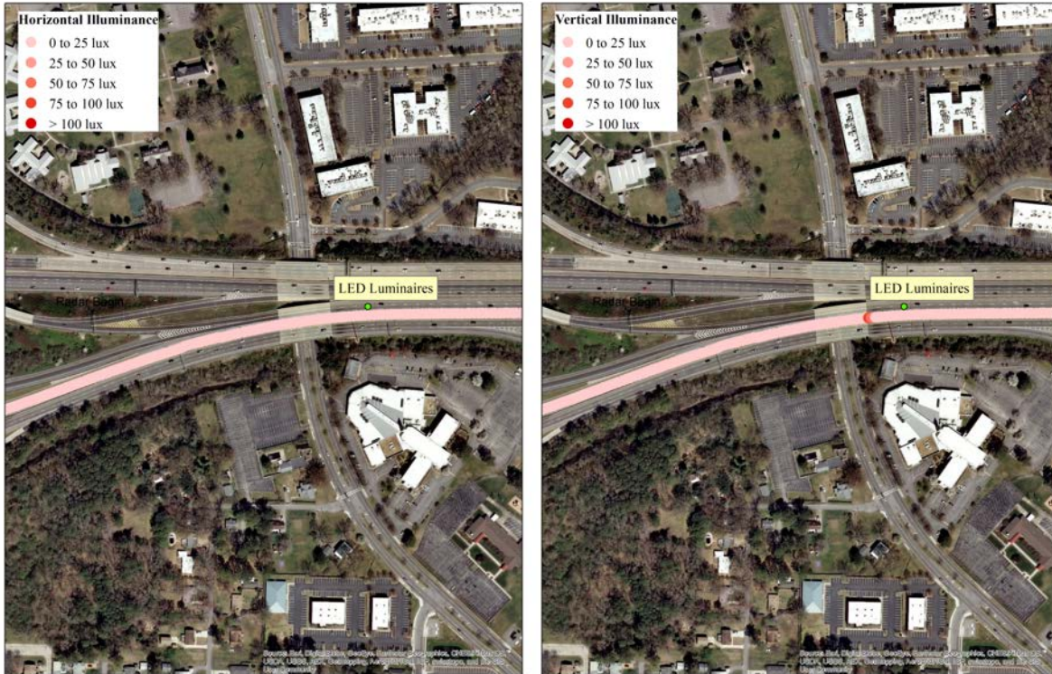
Figure 17. Horizontal and vertical illuminance levels at the milling and paving operation on I-264 west.
