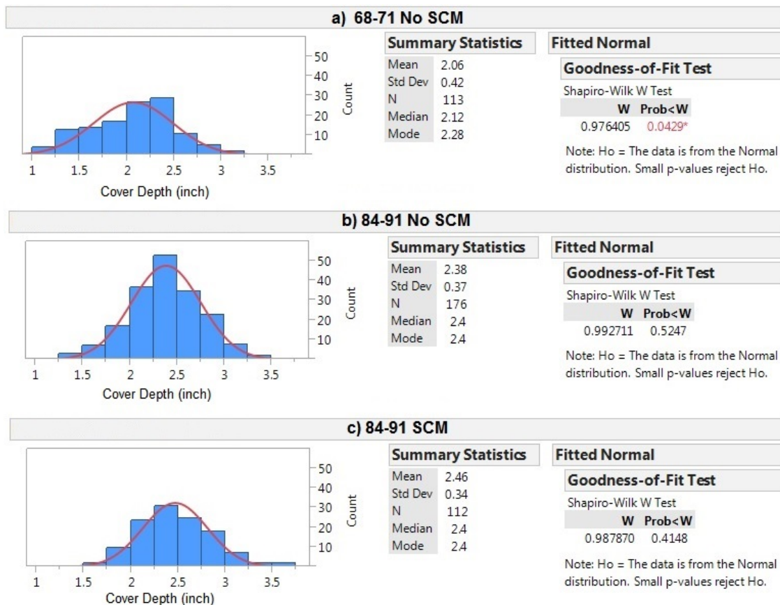
Figure 2. Histograms of Concrete Cover Depths: (a) 1968-71 No-SCM Decks; (b) 1984-91 No-SCM Decks; (c) 1984-91 SCM Decks
