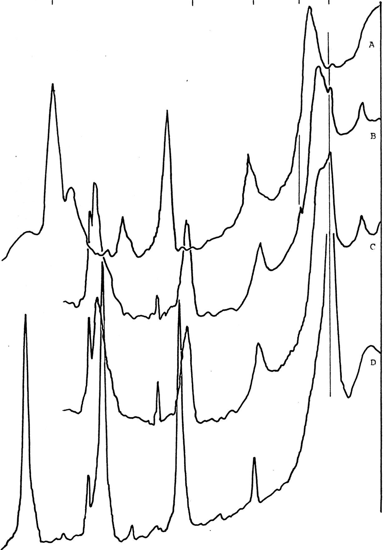
Figure 10—Nason 1C, 5-2 micron fraction, purified, fully expanded by barium chloride treatment, 25 C (A), heated to 110 C (B), and 550 C (C).
