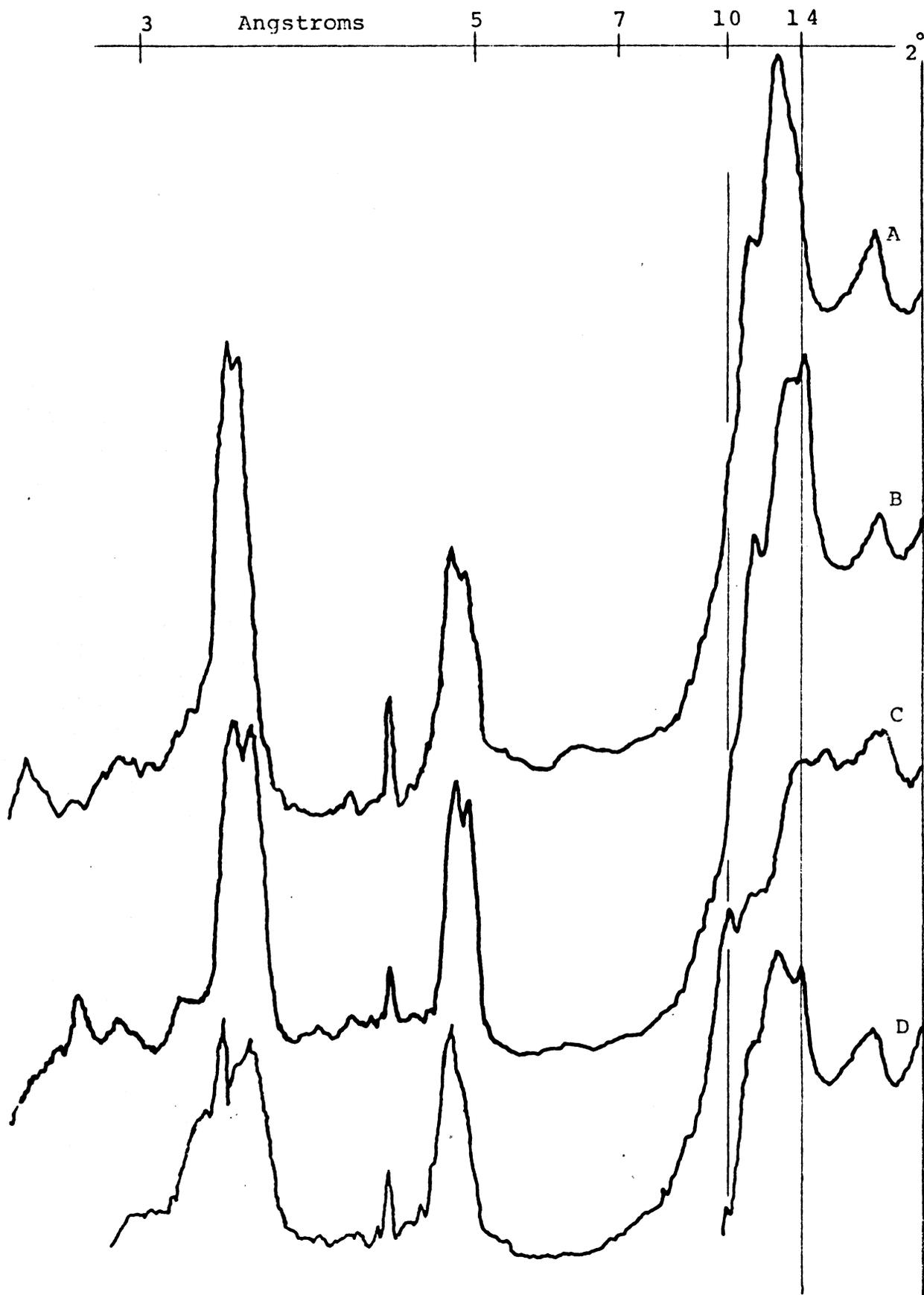
Figure 6—Acid fluoride removal of kaolinite: four day leaching treatment of 5-20 micron Nason IC (A); same sample magnesium saturated (B).
