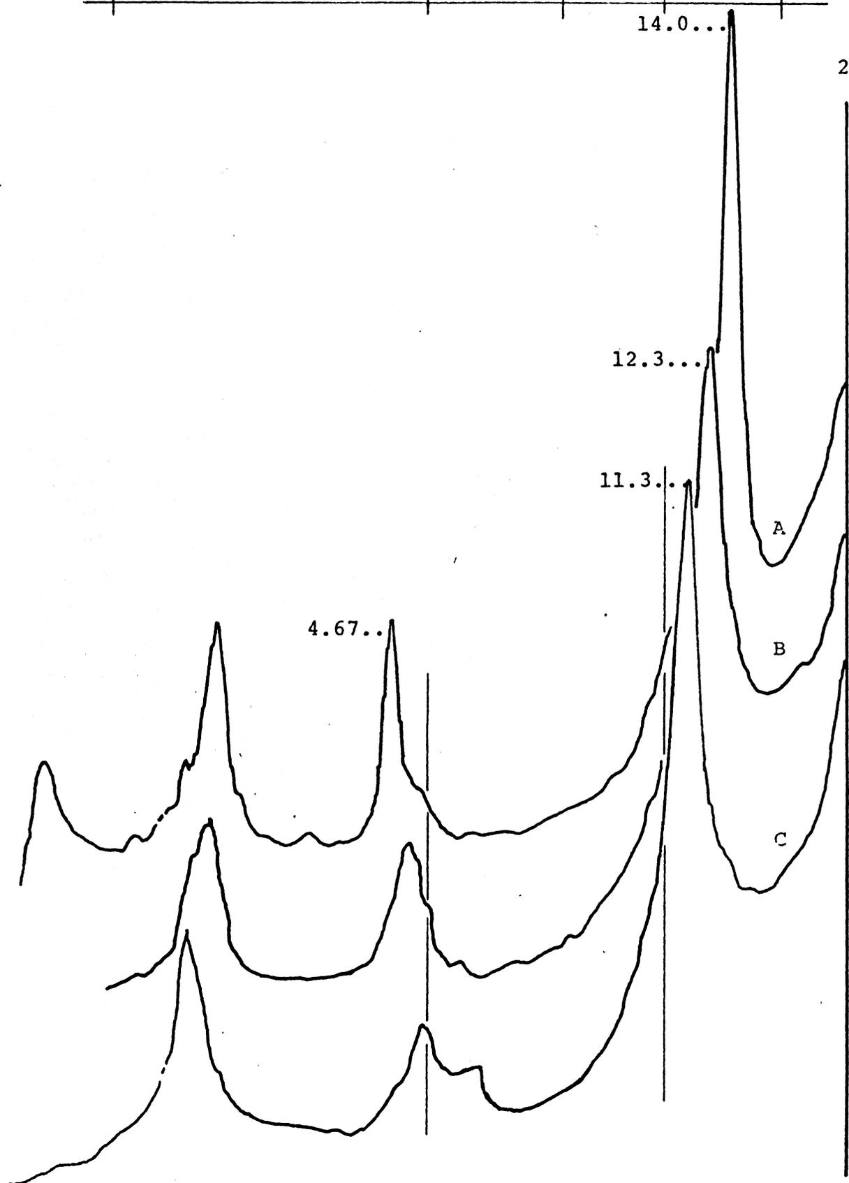
Figure 27—Linearly recorded, x-ray diffractometer pattern of aluminum saturated dioctahedral vermiculite.
