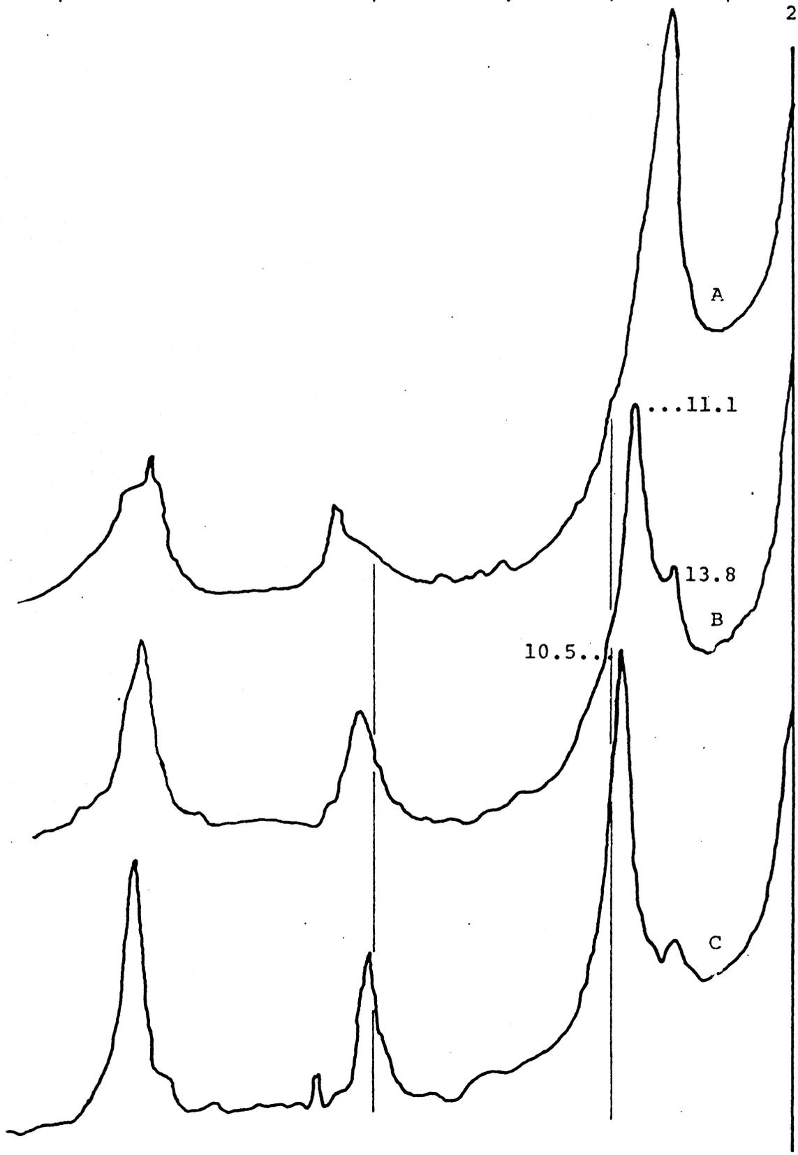
Figure 26—Nason 1C, 5-20 micron fraction, fully expanded Mg-vermiculit aluminum saturated by eight washes, hydrolyzed by two washes, and a 24 hour boiling treatment in solutions with OH/Al ratio equal to 1.75, potassium saturated, 25 C (A), 110 C (B), 300 C (C).
