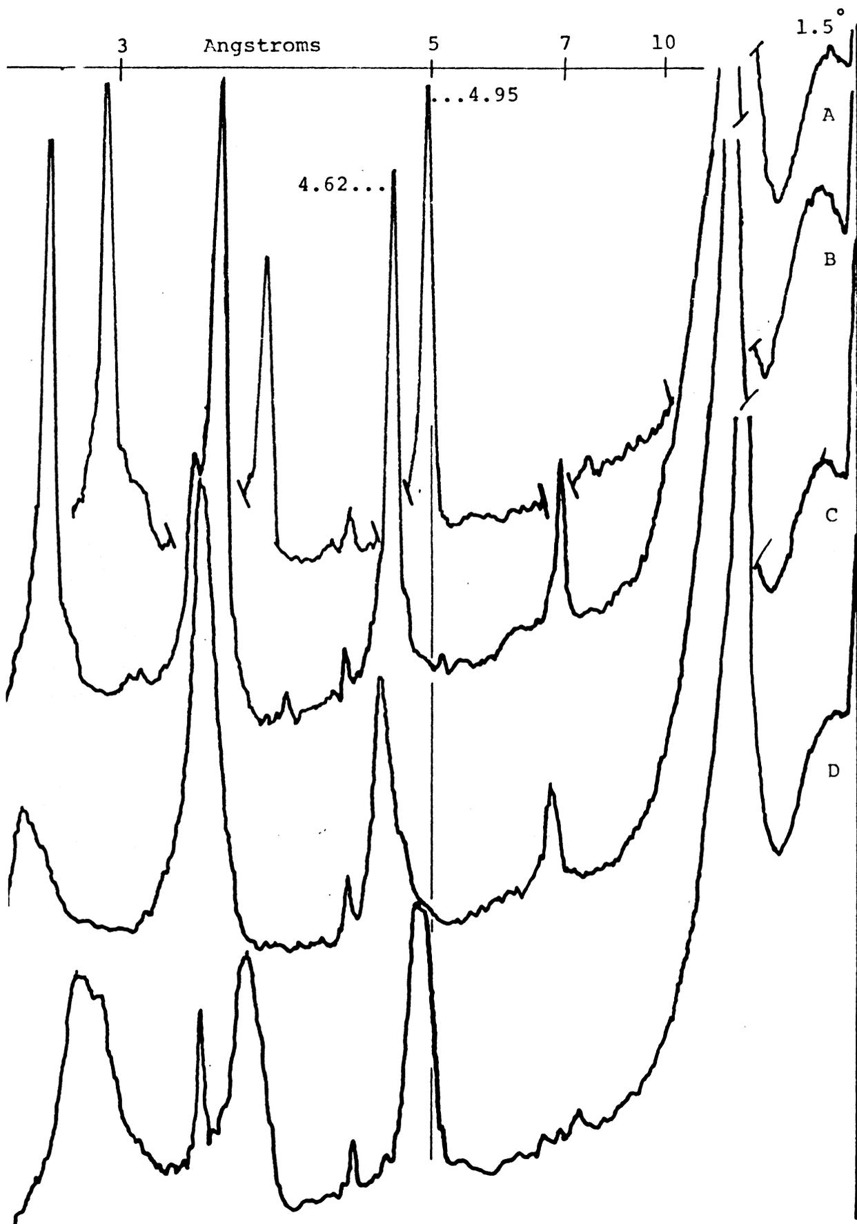
Figure 18—Fully expanded vermiculite derived from Nason 1C, 5-2 micron fraction, magnesium saturated followed by calcium saturation with autoclave treatments air dry, 25 C (A); same sample hydrated at 100 percent relative humidity (B).
