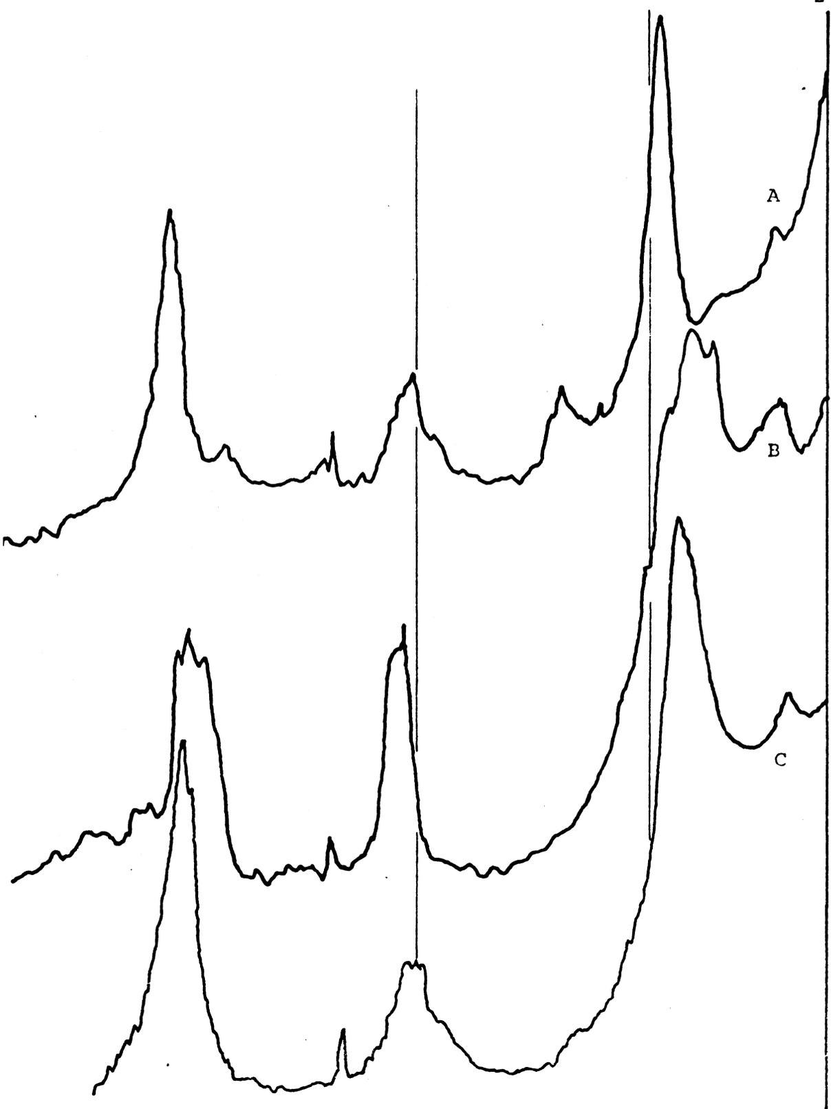
Figure 5—Effect of leaching using sodium citrate on expansion of 5-2 micron magnesium saturated Nason IC after selective dissolution of kaolinite by method of Hashimoto and Jackson: five day treatment (A), ten day treatment (B), ten day treatment glycerol solvated (C), ten day treatment glycerol solvated and heated to 110 C (D).
