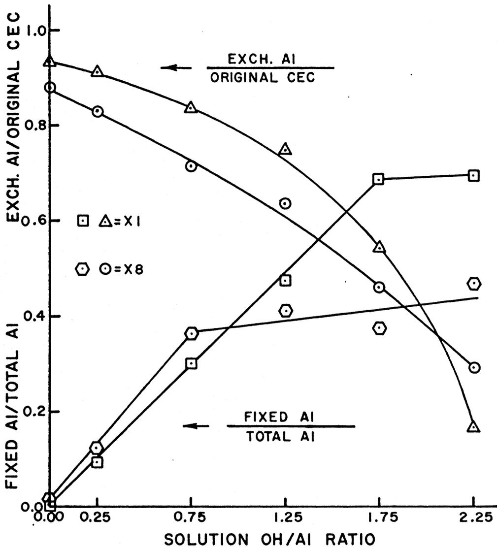
Figure 3—Comparison of decrease in cation exchange capacity in X8 and XI resins saturated with aluminum or potassium after 2 week hydrolysis treatment.
