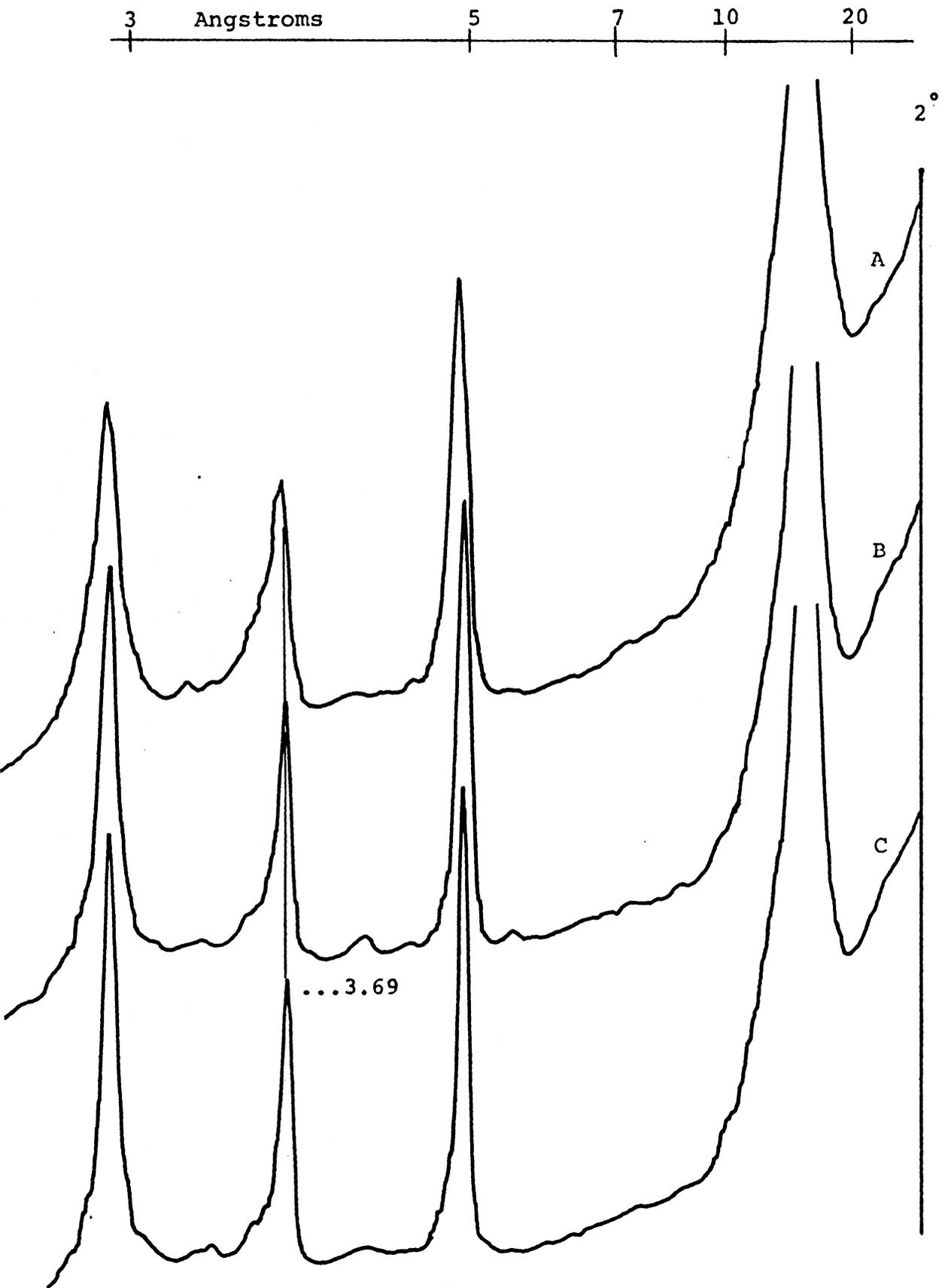
Figure 23—Nason 1C, 5-2 micron fraction, fully expanded vermiculite, aluminum saturated by prolonged single treatment, after hydrolysis and determination of cation exchange capacity (A); same slide after one year storage air dry (B); and hydration at 100% relative humidity (C).
