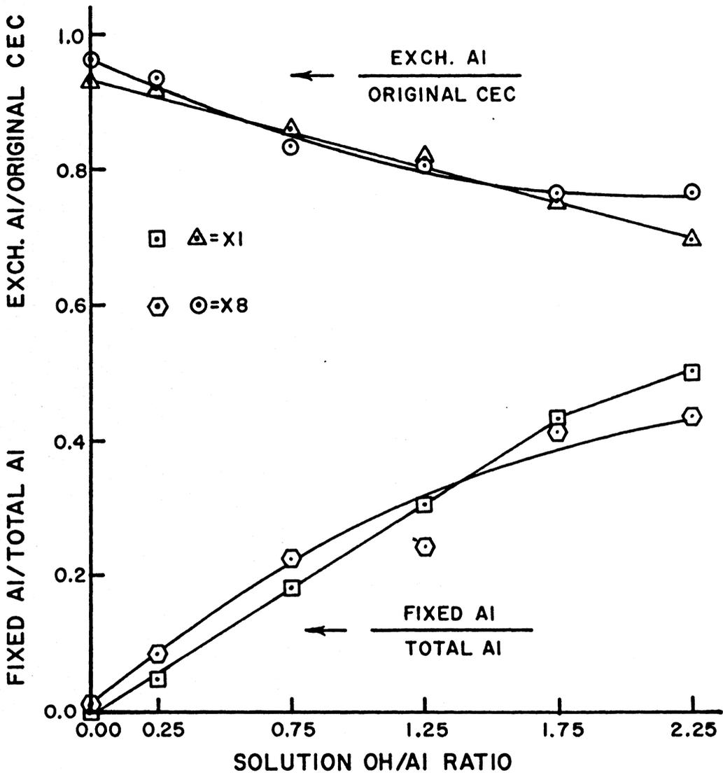
Figure 2—Relationship of fixed aluminum to total aluminum in the system and exchangeable aluminum to original cation exchange capacity in Dowex 50 X8 and X1 potassium saturated resins after two week hydrolysis treatment.
