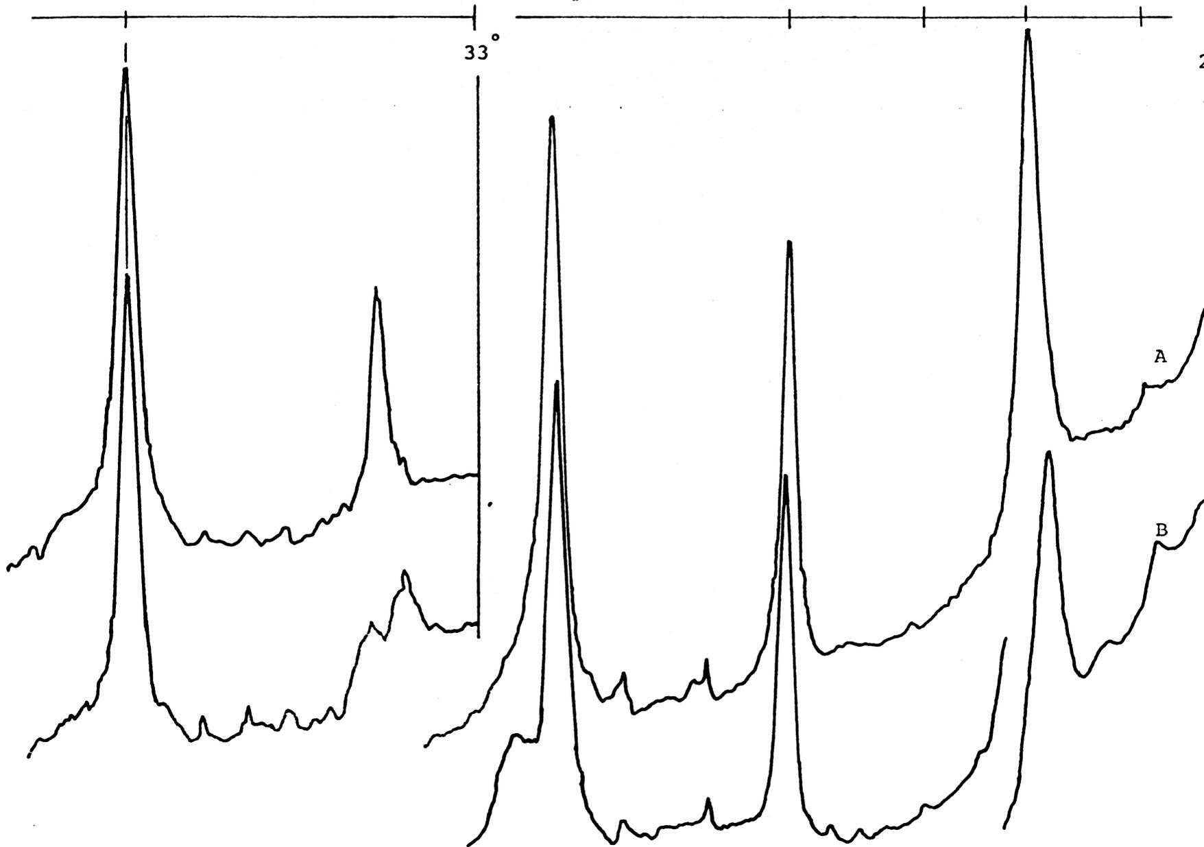
Figure 7—Effect of selective dissolution technique proposed by Hashimoto and Jackson on crystallinity of 5-2 micron Nason IC as seen by sample leached five days by sodium citrate, magnesium saturated, heated to 550 C (A) compared with the sample without prior selective dissolution treatment, heated to 550 C (B).
