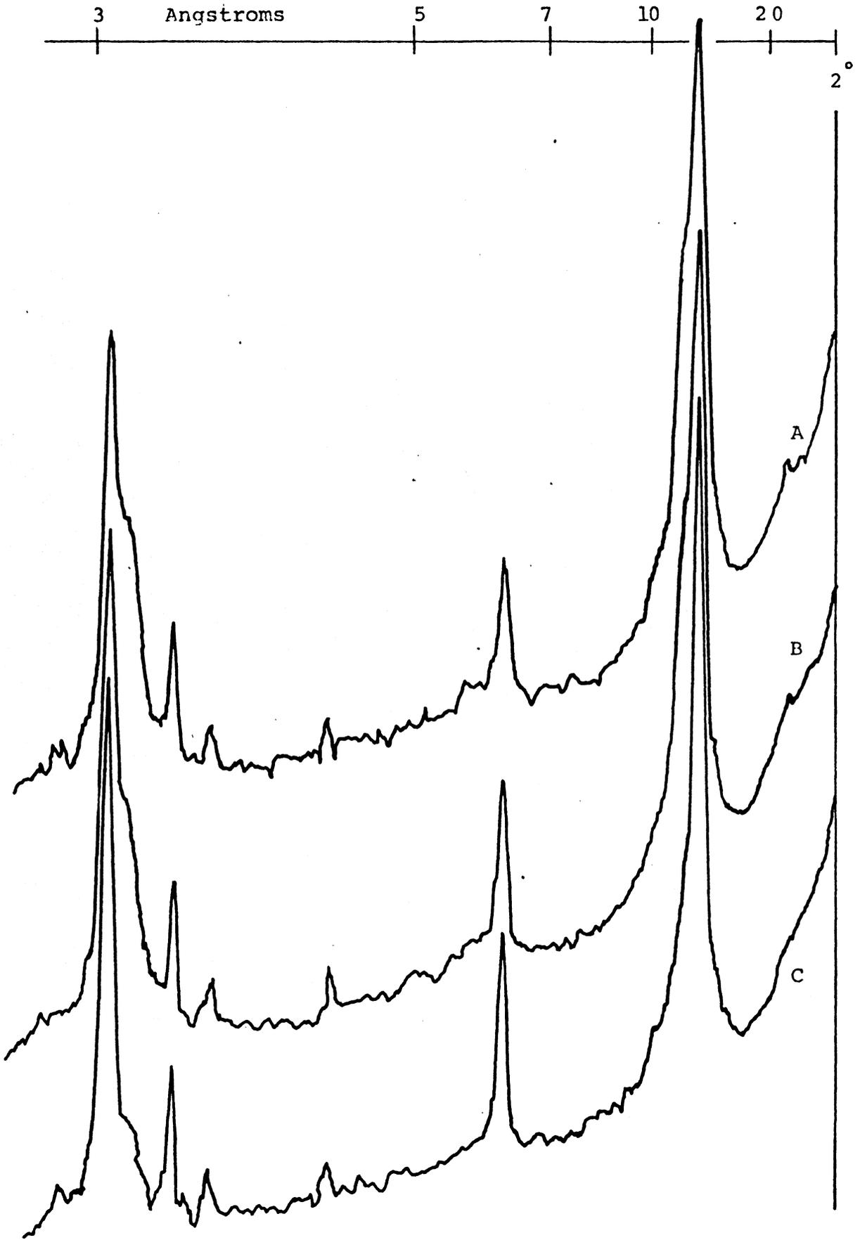
Figure 12—Nason 11C, 5-2 micron fraction, purified, partially expanded by a single barium chloride treatment (A), five barium chloride treatments (B), eight barium chloride treatments (C).
