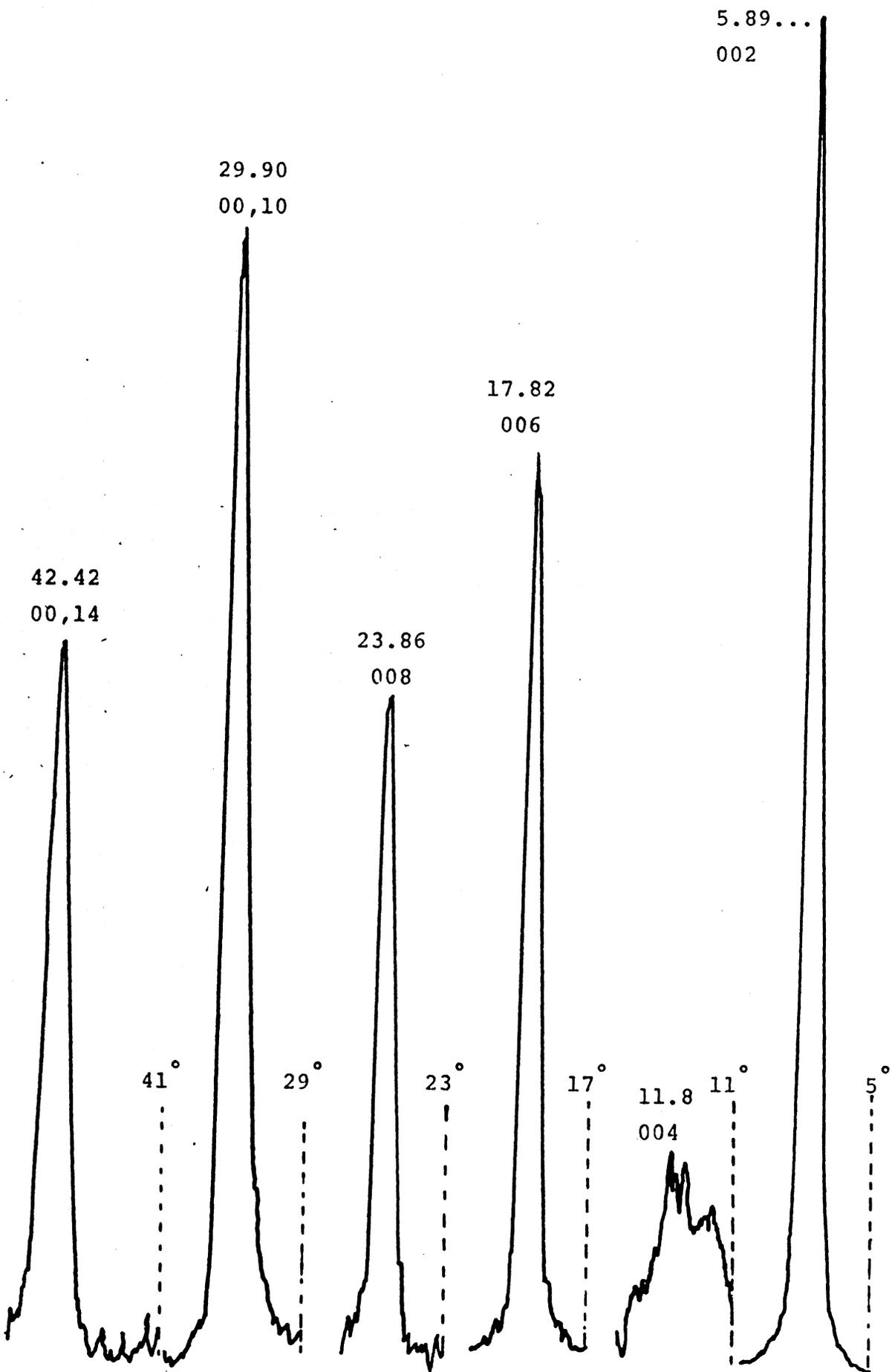
Figure 28—Linearly recorded, x-ray diffractometer pattern for aluminum saturated dioctahedral vermiculite.
