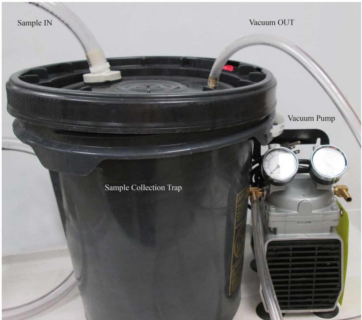
Figure 4.3. Fully assembled custom-made vacuum-assisted collection device used to suction rumen contents out of the rumen and temporarily store rumen contents. See text for specifications.
