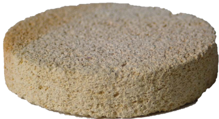
Image 6: Kiln brick cut to the 4" diameter need to be placed in the impedance tube
