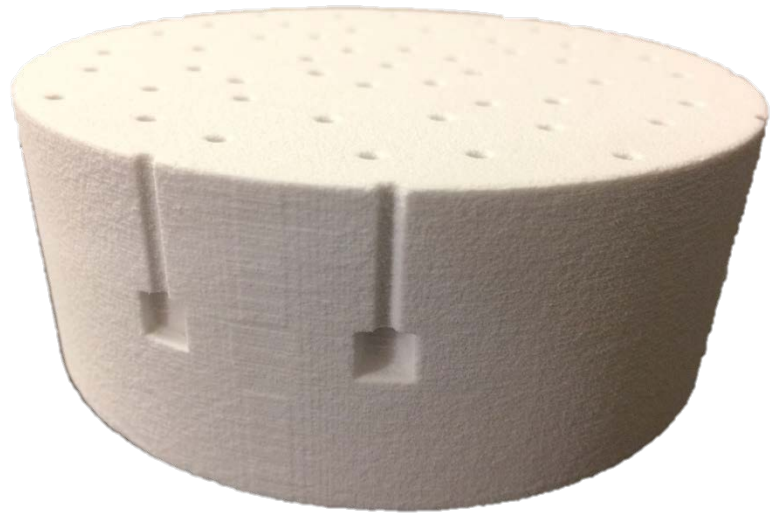
Image 2: Powder based 3D printed cube Helmholtz resonator
