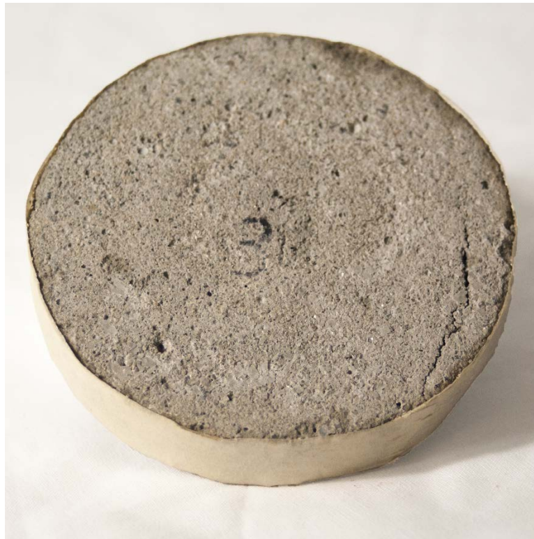
Image 4: Portland cement tile with 1 part cement to 3 parts sand
