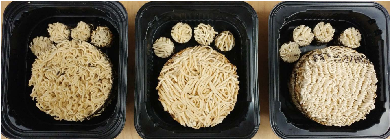
Image 5: Three packaged ramen noodle products cut to fit inside the B&K impedance tube
